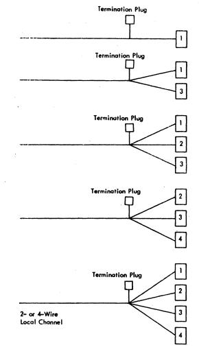
Figure 31. Representive Distributions of Subchannels on a Local Channel
