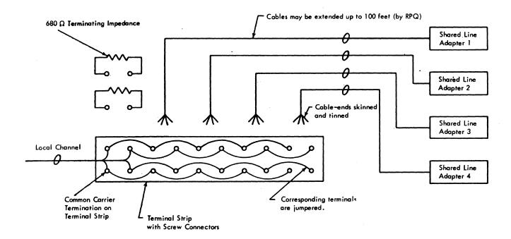
Figure 36. Up to Four Shared Line Adapters Per Local Channel (World Trade)
