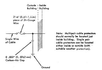
Figure 21. Fuse and Carbon-Air Gap Protection for a Single Wire of a Cable
