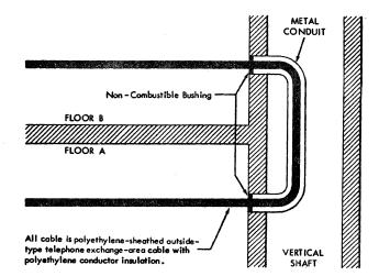
Figure 18. Metal Conduit, Used for Vertical Run Between Floors
