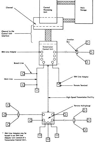
Figure 2. Data Communications System Configuration
