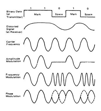
Figure 1. Comparison of Direct Data Transmission and Modulation of a Carrier Frequency
