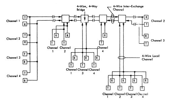
Figure 32. Multipoint Channel, Showing Flexibility of IBM Shared Line Adapter Subchannels
