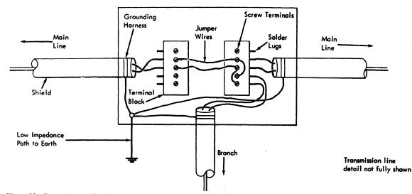
Figure 22. Grounding at a Junction Box
