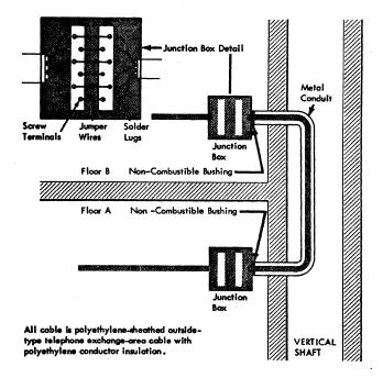
Figure 19. Metal Conduit, Used for Vertical Run Between Junction Boxes
