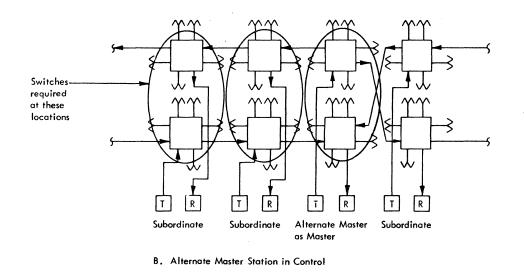
Figure 28. Regular and Alternate Master Station Served from Different Bridges
