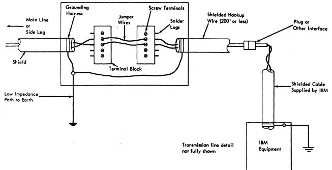
Figure 23. Grounding at a Terminal Box
