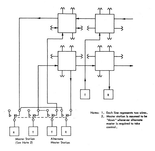
Figure 27. Regular and Alternate Master Station Served from the Same Bridges
