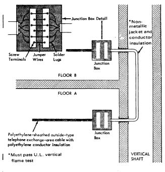
Figure 20. Non-metallic-Jacketed Cable used for Vertical Run Between Junction Boxes
