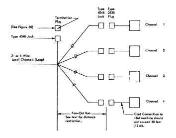
Figure 33. Fan-Out Run for IBM Shared Line Adapter
