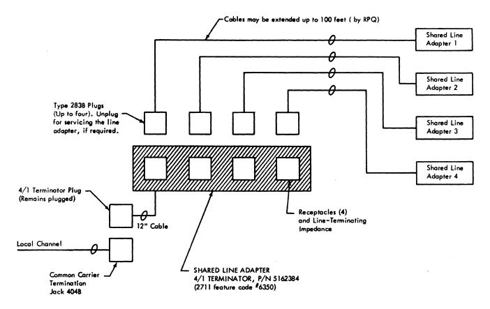
Figure 35. Up to Four Shared Line Adapters Per Local Channel (USA)
