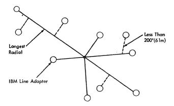
Figure 16. Radial Configuration, for Sample Calculation Using IBM Limited Distanco Line Adapter Type 2
