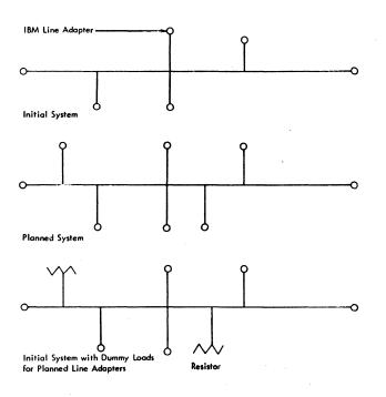
Figure 11. Simulating a Line Adapter with a Dummy Load
