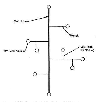
Figure 15. Main Line with Branches, for Sample Calculations Using IBM Limited Distance Line Adapter Type 2 Figure 16 shows a radial configuration, using IBM Limited Distance Line Adapter Type 2.
