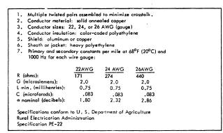
Figure 8. Specifications for Outside-Type Telephone Exchange-Area Cable
