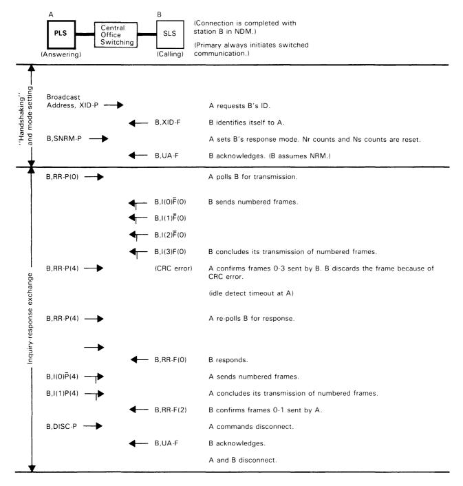
Figure 27. Two-way Alternate Exchanges on Switched Point-to-Point Links
