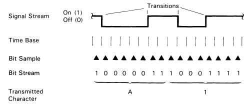
Figure 7. Discrete Transmission Coding
