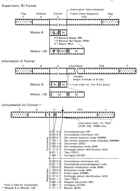
Figure 29. SDLC Frames, As Transmitted
