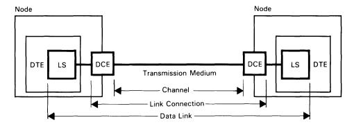
DCE Data Circuit-terminating Equipment
