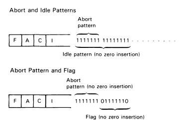
Figure 17. Transmitting Station Aborts Transmission
