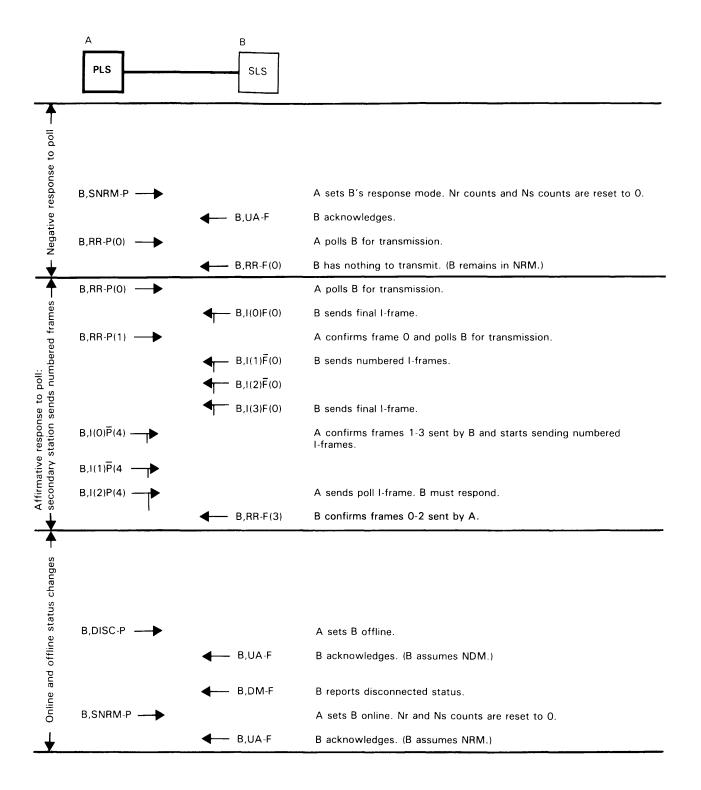
Figure 24 (Part 1 of 2). Two-way Alternate Exchanges on Nonswitched Point-to-Point Links
