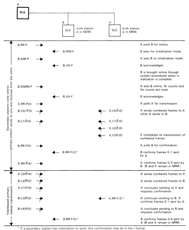
Figure 26. Two-way Simultaneous Exchanges on Nonswitched Multipoint Links
