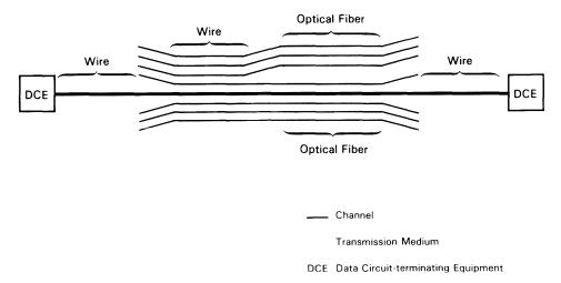
Figure 2. Channels and Transmission Media
