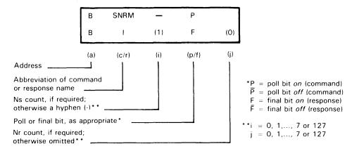
Figure 23. Format of Examples of SDLC Exchanges
