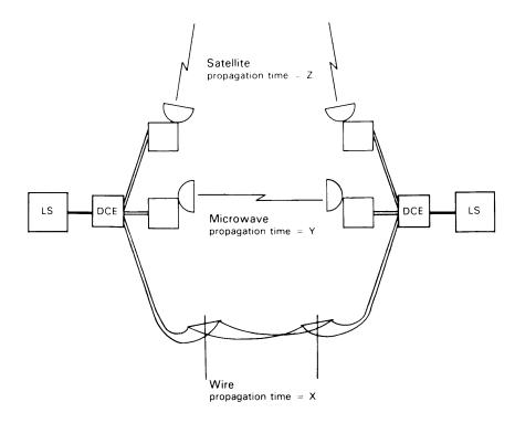
Figure 16. Examples of Telecommunication Facilities
