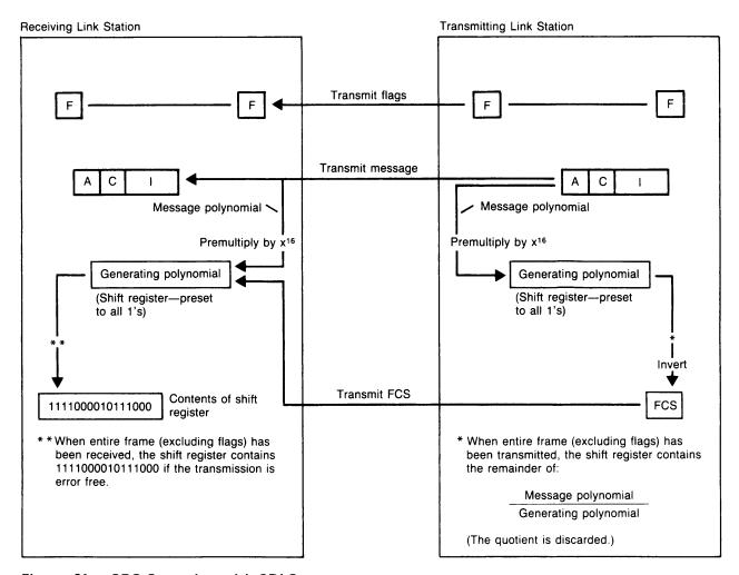
Figure 31. CRC Operation with SDLC
