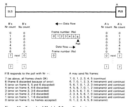
Figure 14. Example of Modulo-8 Frame Numbering
