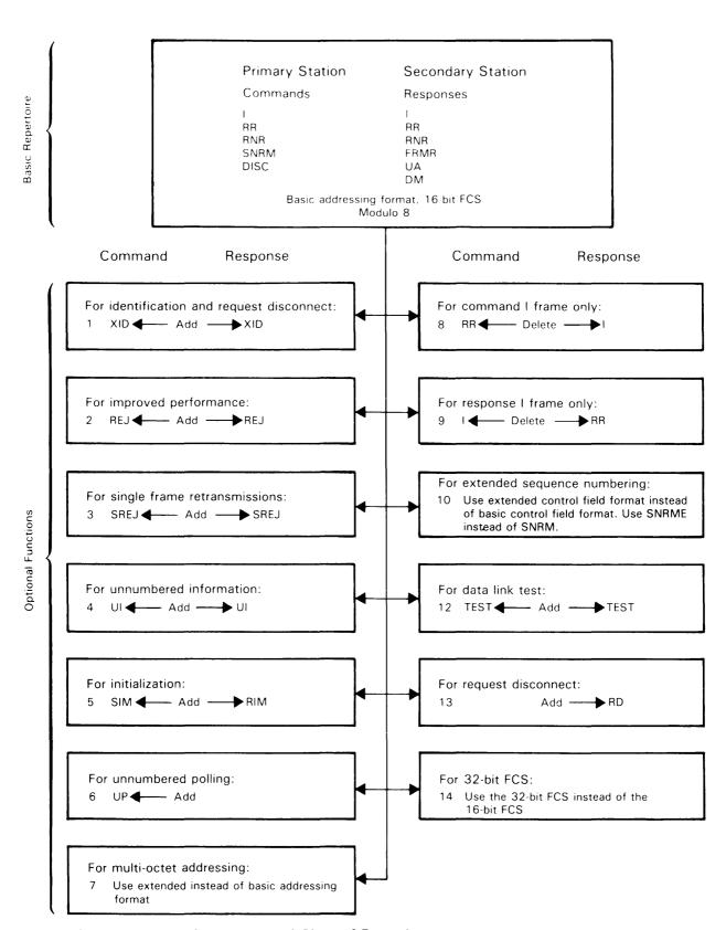
Figure 32. HDLC Unbalanced Normal Class of Procedures
