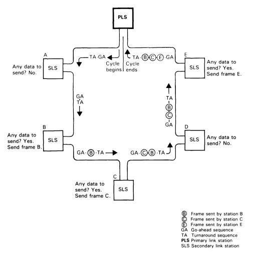
Figure 22. SDLC Loop Exchanges: Secondary Stations Transmitting
