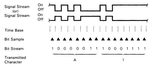
Figure 8. Invert-on-Zero Transmission Coding
