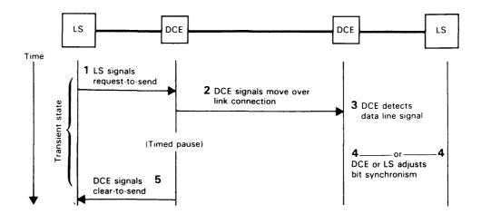
DCE Data Circuit-terminating Equipment LS Link Station
