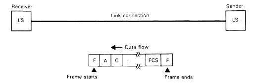
Figure 11. SDLC Transmission Frame
