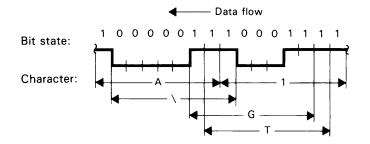
The receiver and the transmitter must be in bit and character synchronism (lack of synchronism results in inability of receiver to determine if incoming character is  $A, \setminus G$ , or T).
