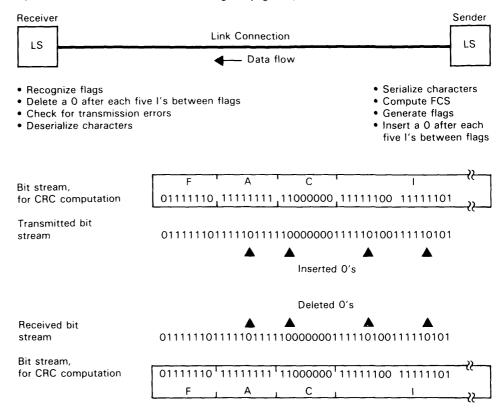
Figure 15. Zero Insertion and Deletion
