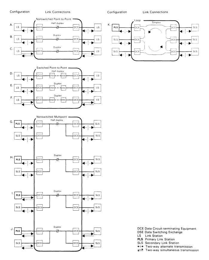
Figure 4. Link Connection Configurations and Link Station Operation
