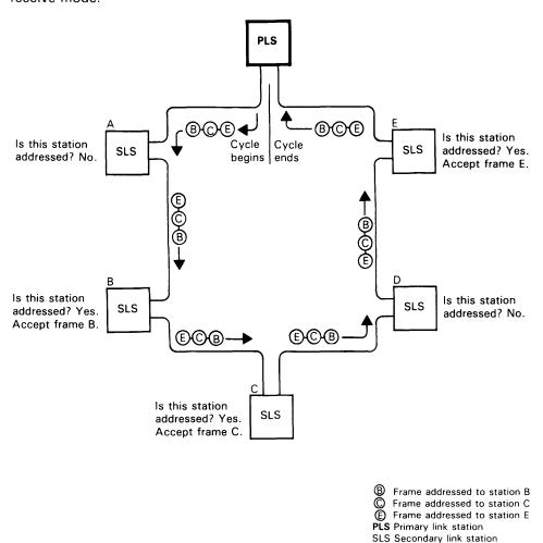
Figure 21. SDLC Loop Exchanges: Primary Station Transmitting
