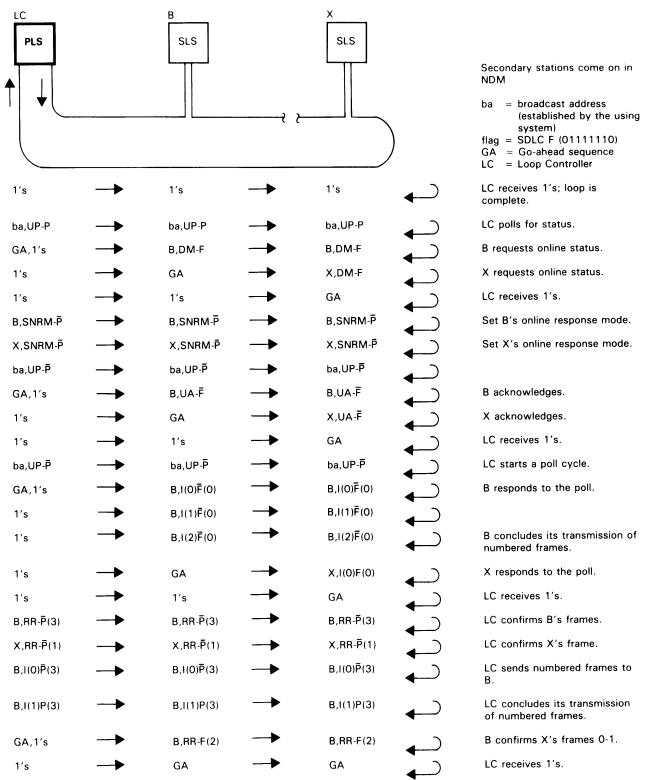
Figure 28 (Part 1 of 2). Two-Way Alternate Exchanges on SDLC Loops
