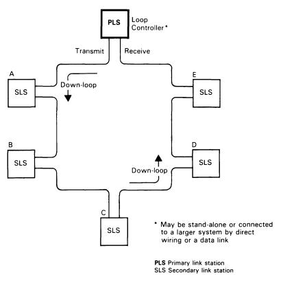
Figure 20. Loop Configuration
