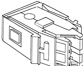
Figure 3-4: Medium Interface Connector
