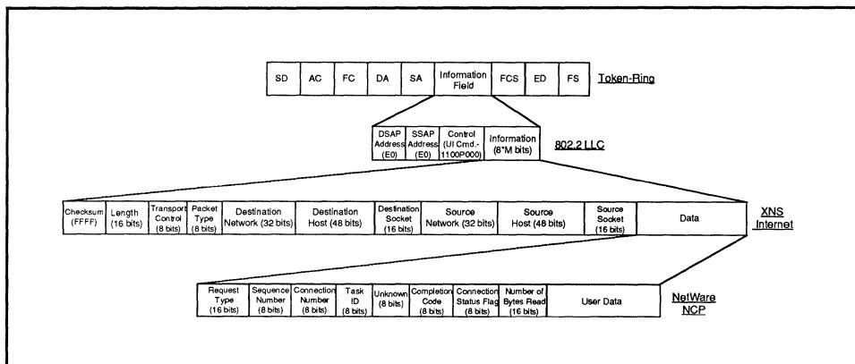
Figure 7-7: Encapsulated NetWare Protocols
