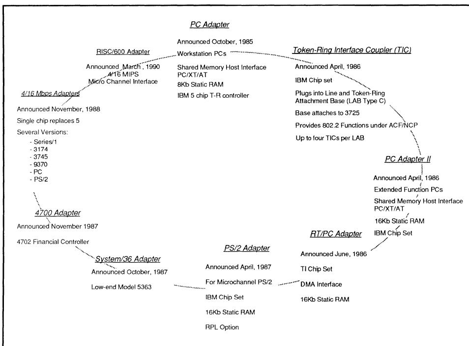
Figure 2-15: IBM Token-Ring Adapter Evolution
