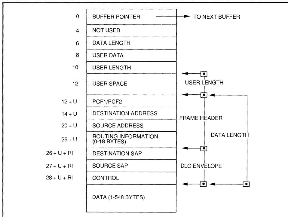
Figure 4-7: Transmit Buffer
