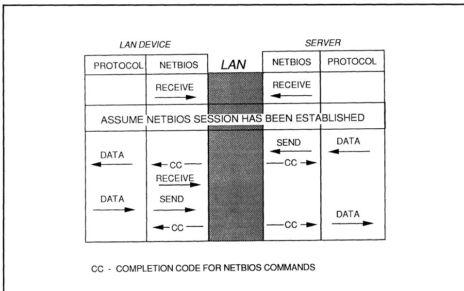
Figure 5-6: Data Transfer ACS Command Flows
