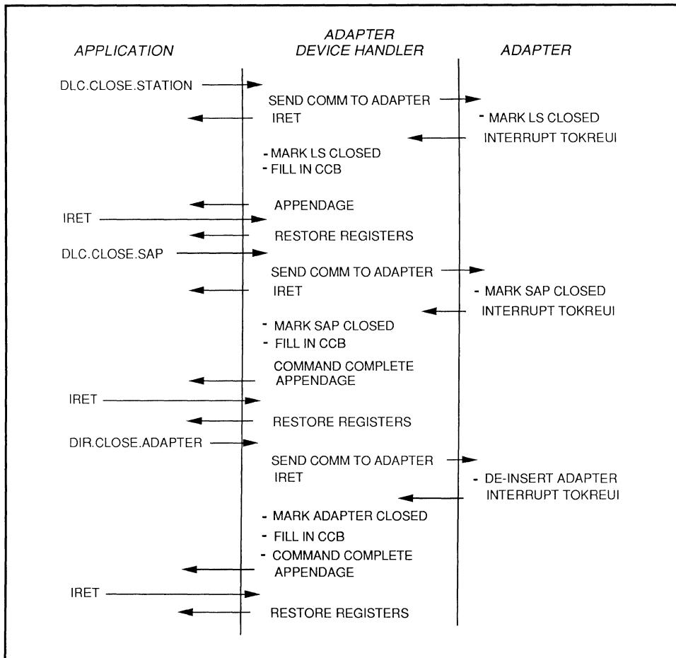
Figure 4-12: Token Handler Command Flow - Shut Down
