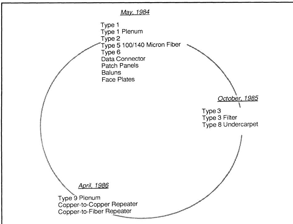
Figure 2-8: IBM Cabling System Evolution
