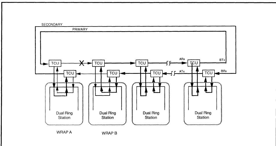
Figure 3-13: Dual Ring Failure Recovery
