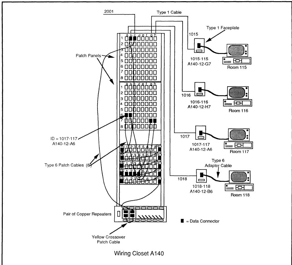
Figure 2-5: MAU Rack Configuration with Repeater
