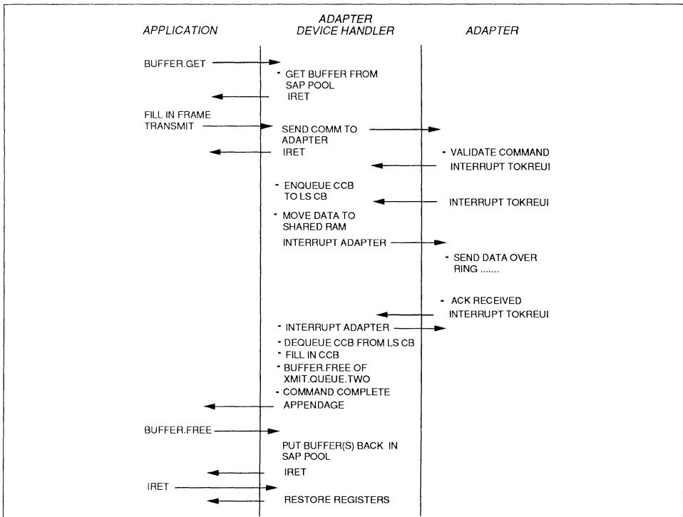
Figure 4-10: Token Handler Cmd Flow - Transmit Data
