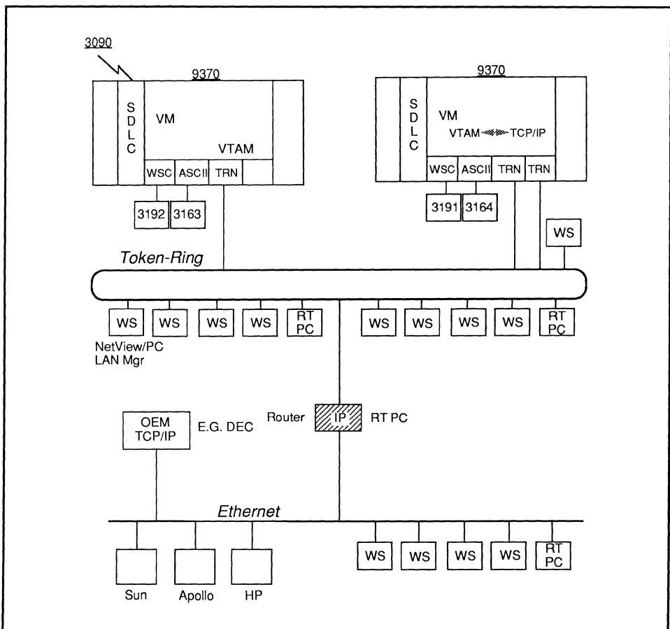
Figure 5-11: 9370: Ethernet to Token-Ring via TCP/IP
