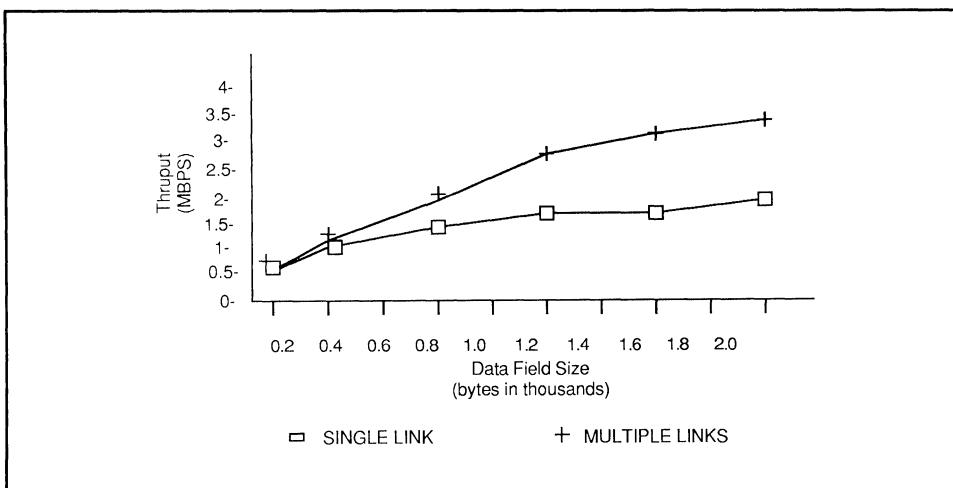
Figure 8-2: Ring Throughput for PC AT
