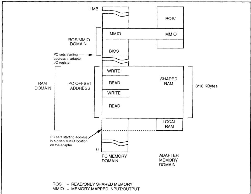
Figure 2-10: Token-Ring PC Adapter Memory Structure
