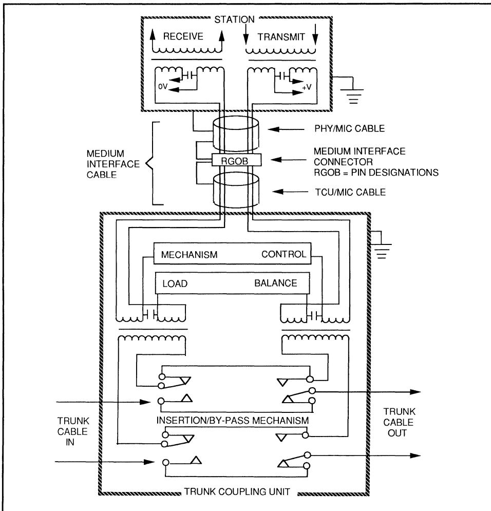
Figure 3-3: Physical Medium Connection Detail
