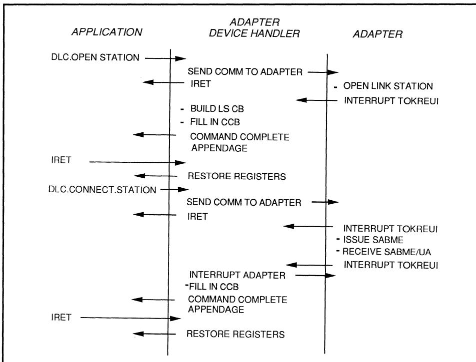
Figure 4-9: Token Handler Flow - Link Connection
