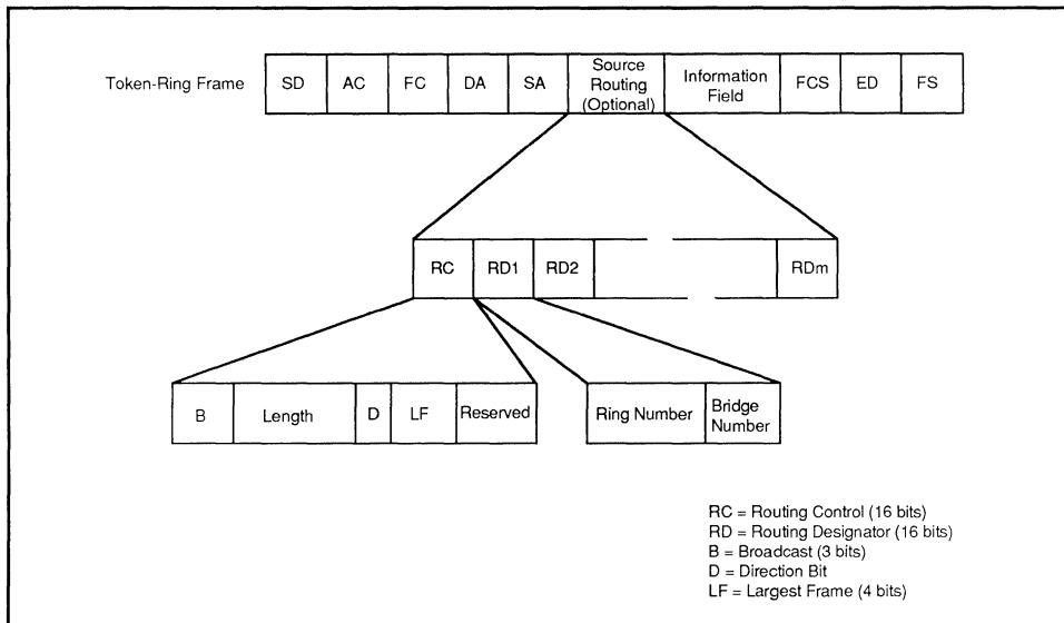
Figure 3-10: Source Routing Field
