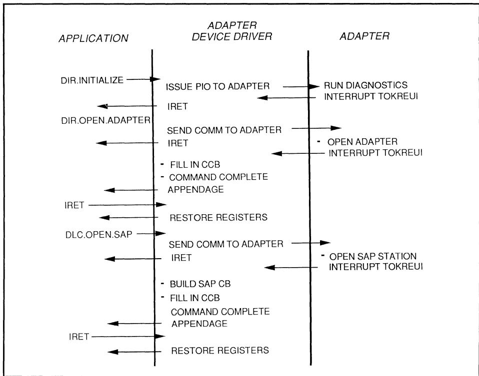
Figure 4-8: Token Handler Command Flow - Starting Up
