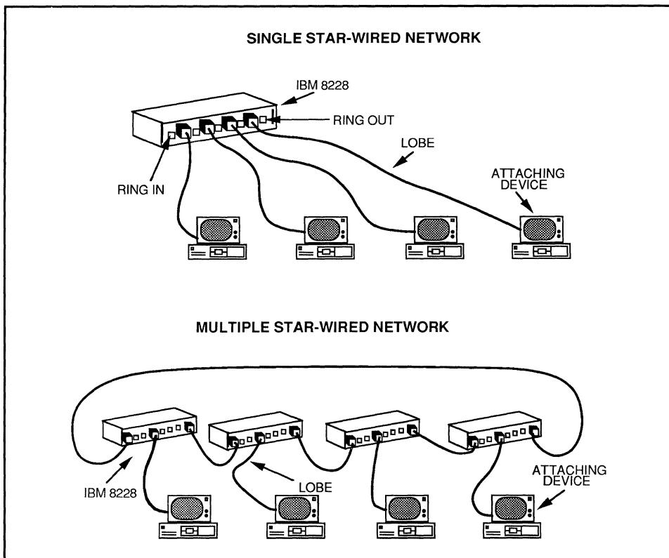
Figure 2-4: MAU Configurations
