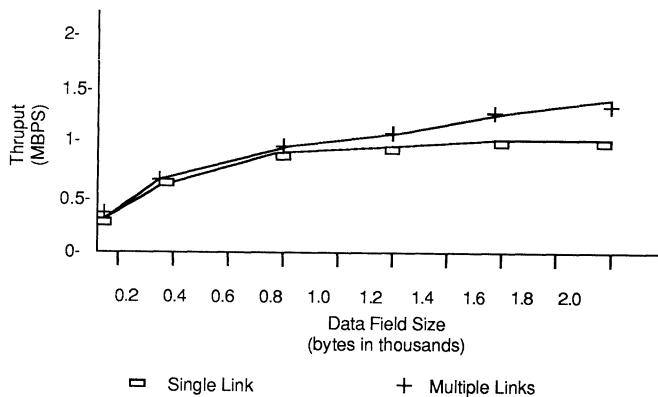
Figure 8-1: Ring Throughput for PC XT
