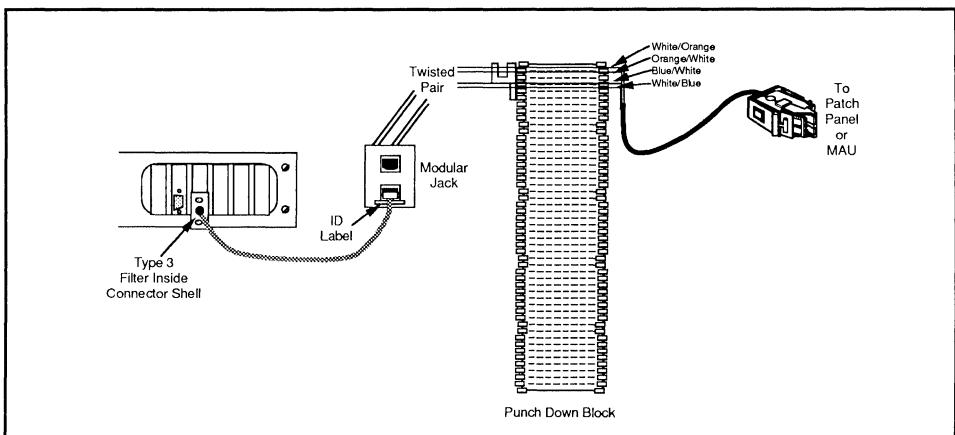
Figure 2-1: Type 3 Wiring Components
