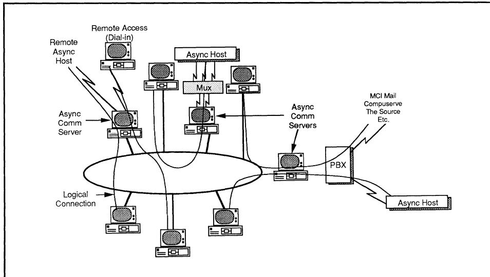
Figure 5-3: Asynchronous Communication Server
