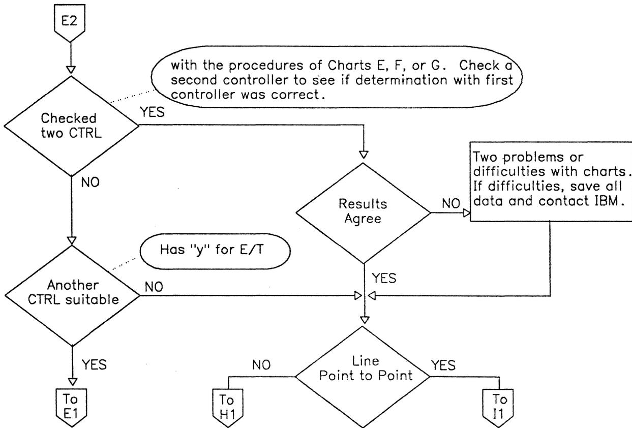
Figure 10. Chart E - Open Line and Initial Line Side (continued)
