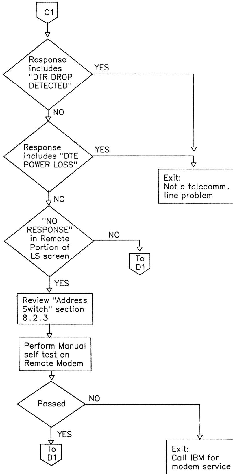
Figure 7. Chart C - LS Test Final Screening
