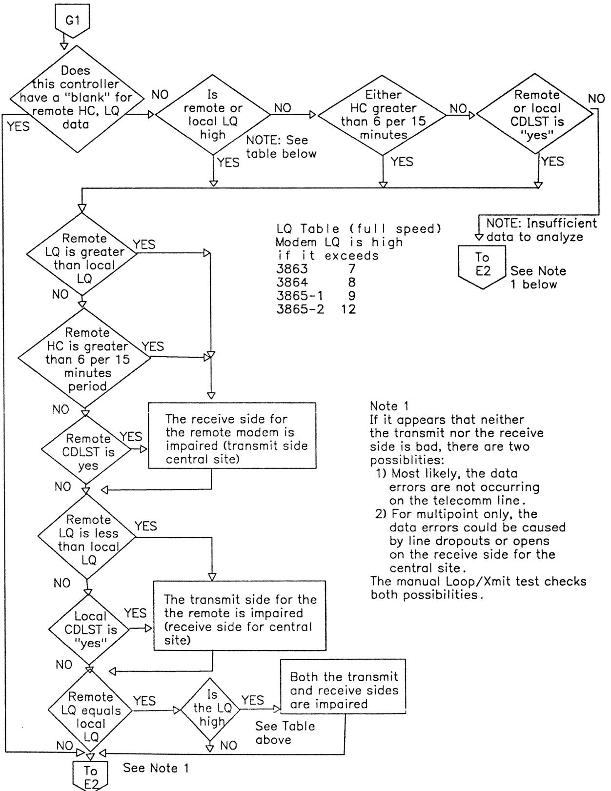
Figure 13. Chart G - Line Direction/Side without "Normal" Data
