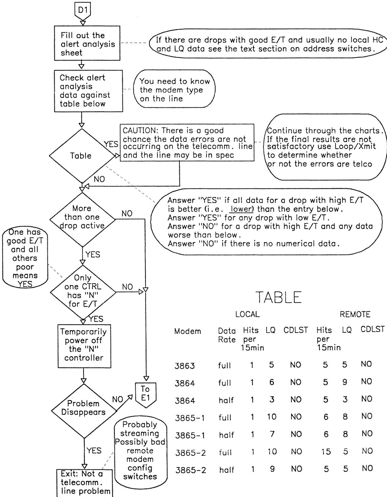
Figure 8. Chart D - Streaming and Initial Line Screening
