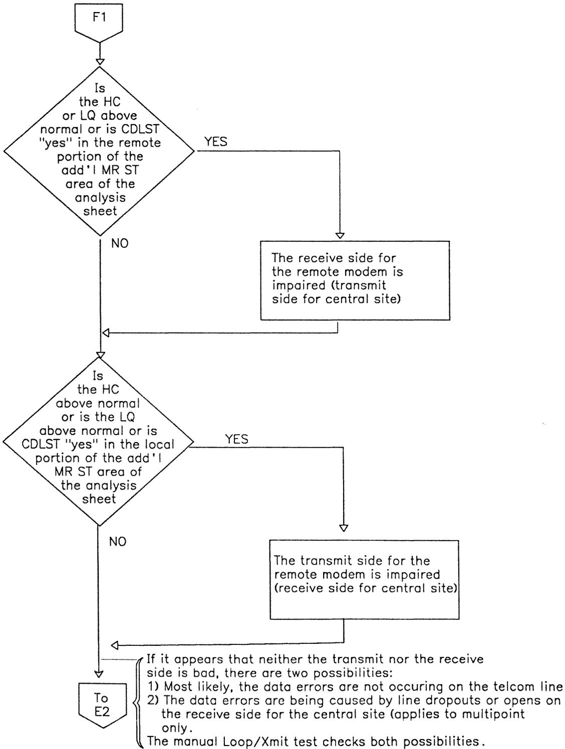
Figure 12. Chart F - Line Direction/Side with "Normal" Data
