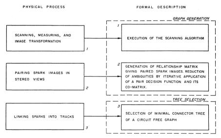
FIGURE 7. Schematic of the relationship of physical processes to formal description
