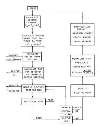
FIGURE 3. Schematic flow chart of first program run on the system depicted by Figure 2
