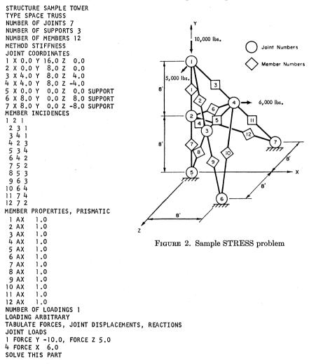
The advantage of such an approach is not just that any structure can be conveniently analyzed, but that any portion of the structure can be singled out for modification by the STRESS-vocabulary words ADDITIONS, DELETIONS, and CHANGES. This facility, especially in a time-shared environment, brings us quite close to the crucial attribute mentioned earlier, namely, that the system output provides meaningful measures of the engineer's decisions.
