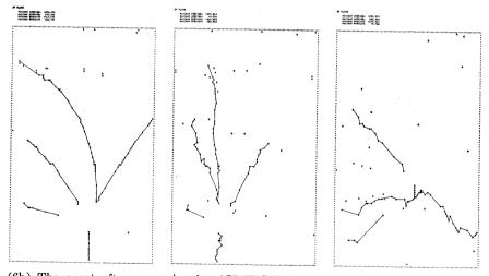
(6b) The event after processing by AIRWICK, showing the reconstructed tracks. Random sparks not on the tracks have now been eliminated.
