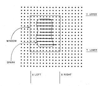
FIGURE 8. Line segments and cells generated by CELL CONSTRUCTION ALGORITHM
