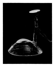
FIGURE 8. Contact lens used for eye-movement recording
