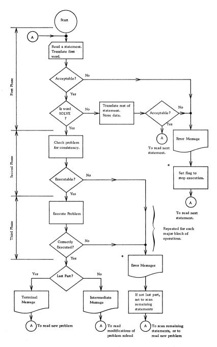
FIGURE 4. Simplified flow diagram of STRESS
