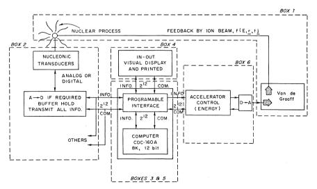
FIGURE 2. Closed-loop analysis and control system being utilized in low-energy nuclear physics experiments
