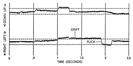
FIGURE 11. Eye movements during fixation. The pairs of horizontal dotted lines represent displacements of 6 minutes arc
