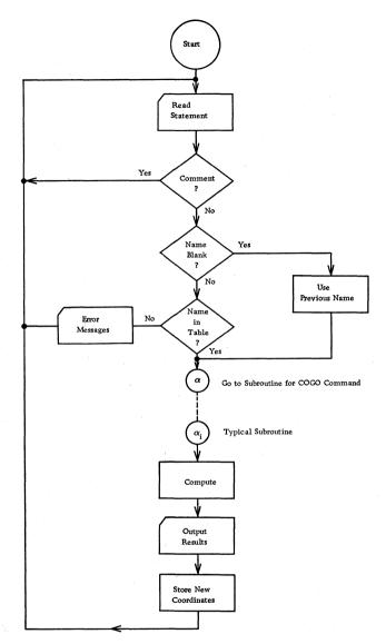
FIGURE 3. Simplified flow diagram of COGO
