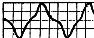
Fig. A. Input from sync track 5 V/CM 20 usec/CM @ 0 volts
