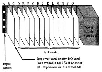
Note. An optional communications power feature provides ±12 volts and is a prerequisite for the following I/O feature cards:
