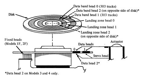
Figure 3-2. Disk and access mechanism
