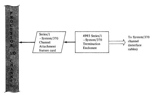
Figure 8-2. Block diagram of 4993 Series/1—System/370 Termination Enclosure
