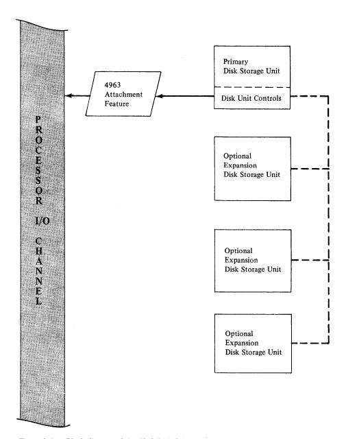
Figure 3-4. Block diagram of the 4963 Disk Subsystem
