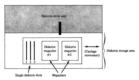
Figure 3-9. Block diagram of the 4966 Diskette Magazine Unit (top view)
