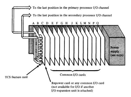
Note. An optional communications power feature provides  $\pm 12$  volts and is a prerequisite for the following I/O feature cards:
