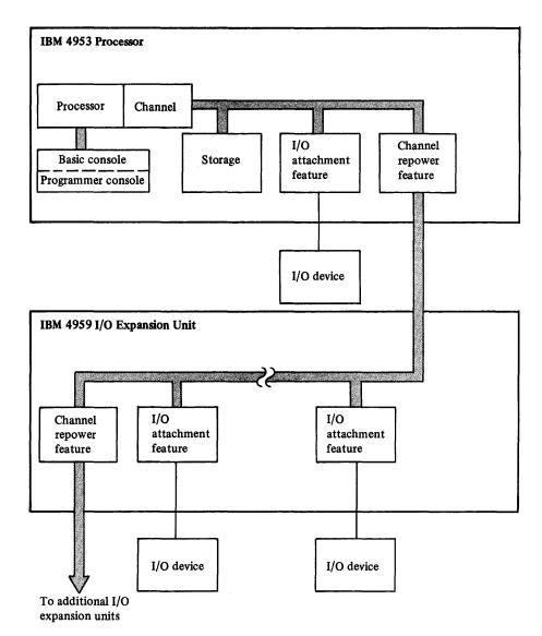
Figure 2-7. Block diagram of a 4953 Processor and a 4959 Input/Output Expansion Unit
