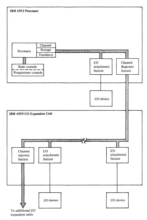
Block diagram of a 4952 Processor and a 4959 Input/Output Expansion Unit
