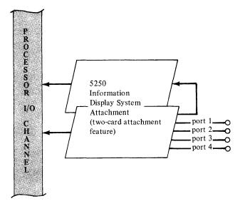
Figure 8-5. 5250 Information Display System Attachment feature
