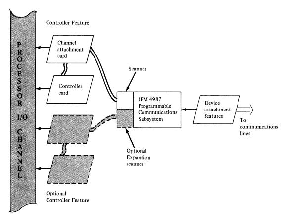
Figure 7-5. Block diagram of a 4987 Programmable Communications Subsystem
