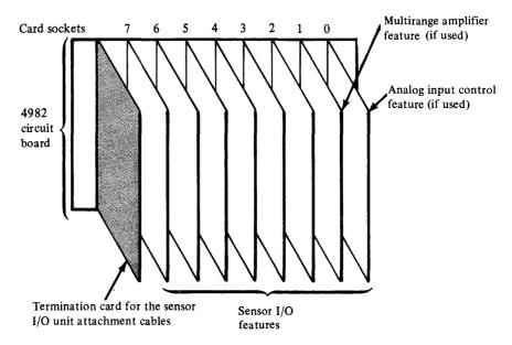
Figure 5-3. 4982 Sensor I/O Unit card sockets (rear view)
