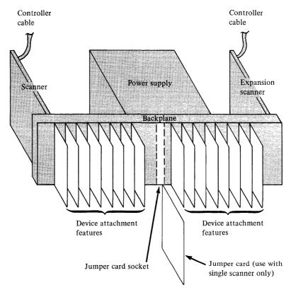
Figure 7-6. 4987 device attachment feature card sockets (rear view)
