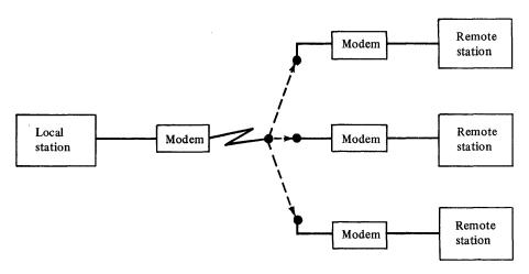
Figure 7-2. Point-to-point switched data link
