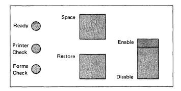
Figure 4-2. Line printer console
