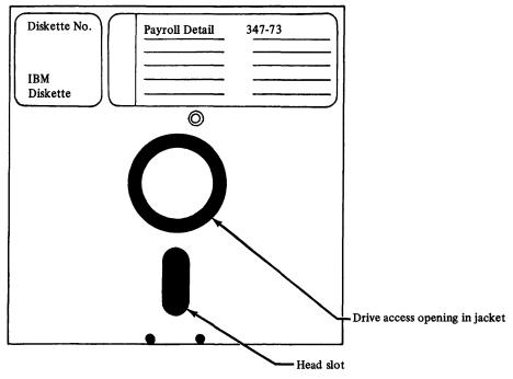
The head slot exposes the recording surface of the disk as the disk turns in its jacket in the machine.
