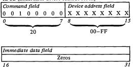
After execution of the Read ID command, the immediate data field of the IDCB contains:
