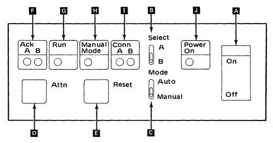
Figure 3-1. TCS Console Controls and Indicators.
