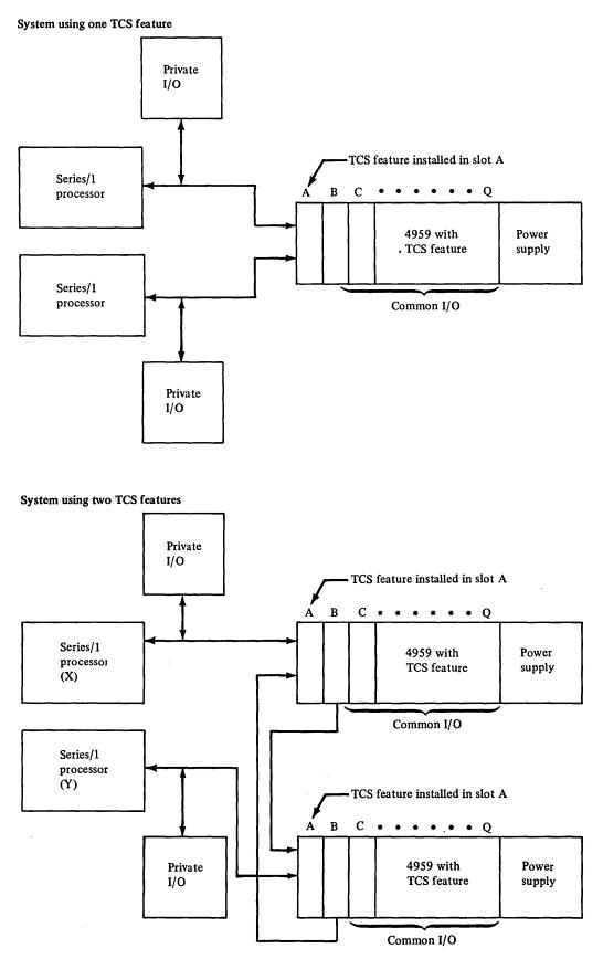
Figure 1-3. Typical system configurations using TCS feature
