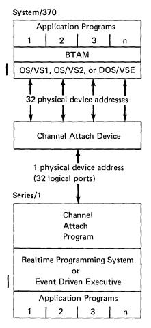
Figure 5-1. A Series/1—System/370 Channel Attach System
