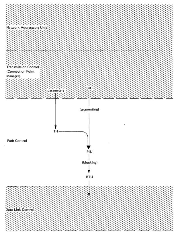
Figure 2-9. Path Information Unit (PIU) and Basic Transmission Unit (BTU)
