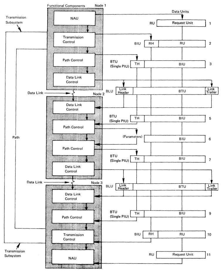
Figure 2-12. Transmission Subsystem Control Data Flow
