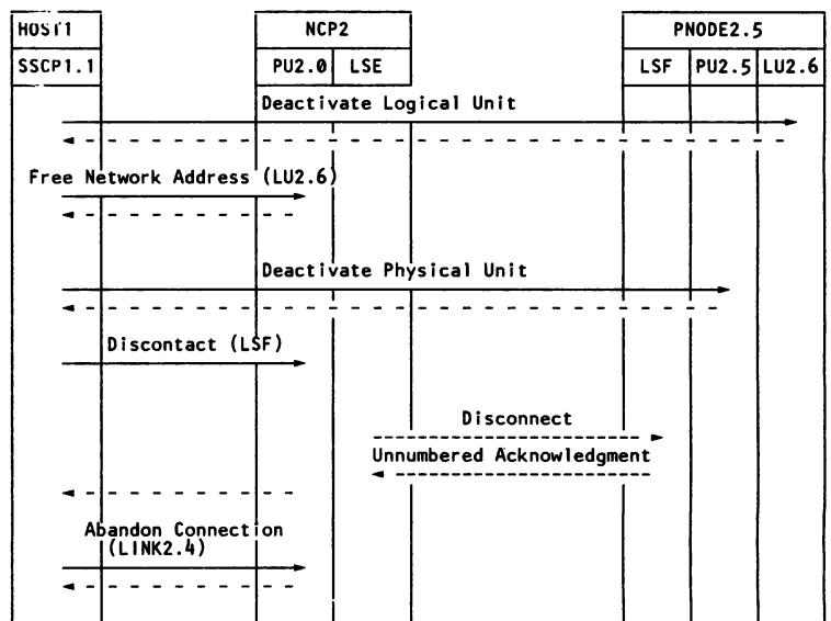
Deactivating a Peripheral Node Attached via a Switched SDLC Link
