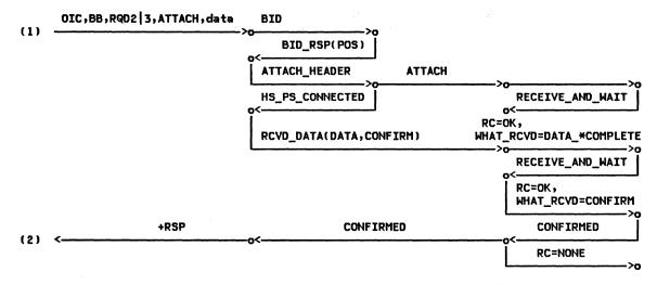
Figure 2-40. ALLOCATE (delayed), CONFIRM (by First Speaker) -- Remote LU
