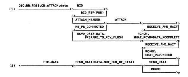
Figure 2-48. ALLOCATE (delayed), RECEIVE\_AND\_WAIT (by Bidder) -- Remote LU
