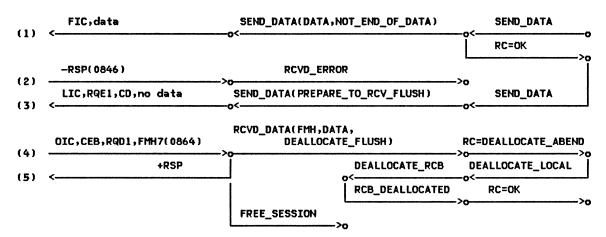
Figure 2-80. DEALLOCATE ABEND Issued in RCV, In-Chain State -- Remote LU
