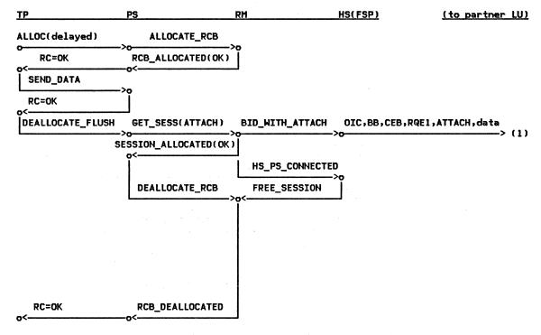
Figure 2-81. ALLOCATE (delayed), DEALLOCATE FLUSH (by First Speaker) -- Local LU
