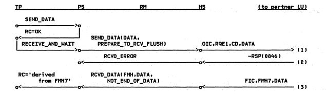
Figure 2-105. SEND\_ERROR at End-of-Chain --Remote LU
