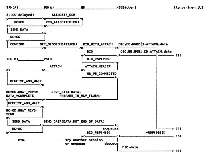
Figure 2-55. ALLOCATE (delayed) Race, Bracket Rejected -- Bidder LU
