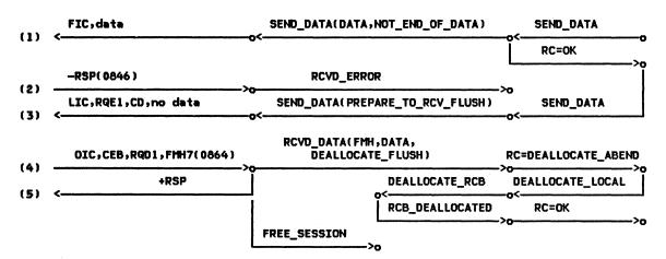
Figure 2-78. DEALLOCATE ABEND Issued in RCV, Between-Chain State -- Remote LU
