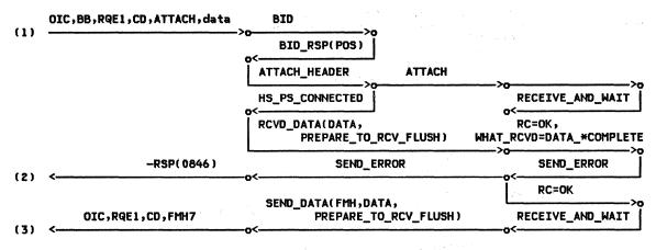
Figure 2-42. ALLOCATE (delayed), RECEIVE\_AND\_WAIT (by First Speaker) -- Remote LU
