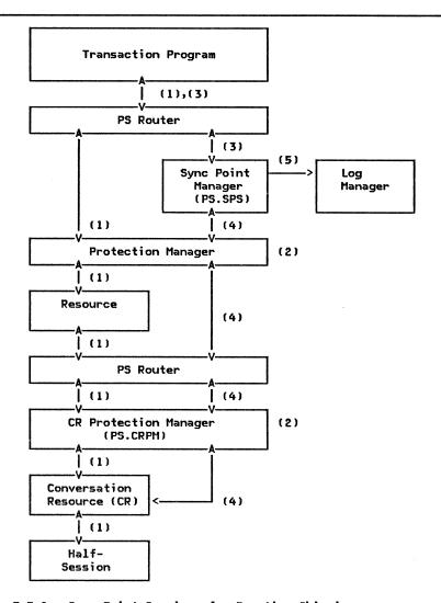
Figure 5.3-8. Sync Point Services for Function Shipping
