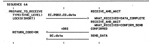
Figure 2-11. Conversation Turnaround with Confirmation, using LOCKS(SHORT):
