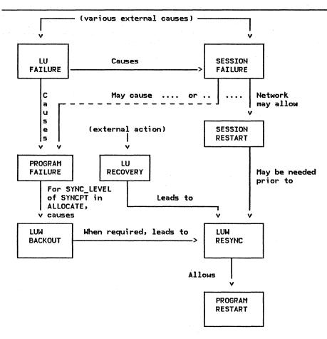
Figure 5.3-1. Relationships among Failures and Recovery
