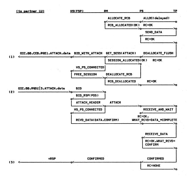
Figure 2-58. ALLOCATE (delayed) Race, Bracket Accepted --First Speaker LU
