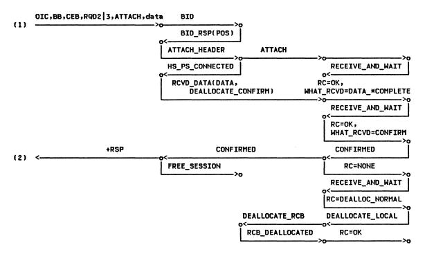
Figure 2-84. ALLOCATE (delayed), DEALLOCATE CONFIRM (BY First Speaker) -- Remote LU
