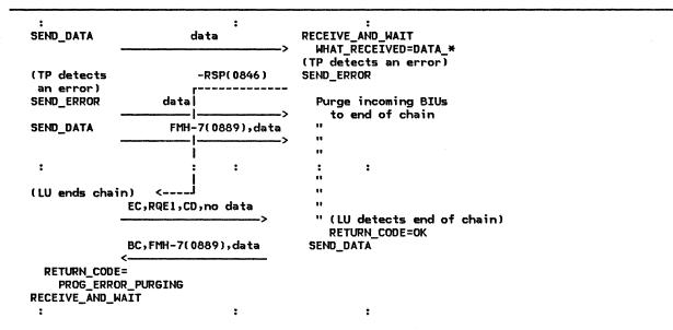
Figure 2-20. SEND\_ERROR Issued by both Sender and Receiver (SEND\_ERROR Race):
