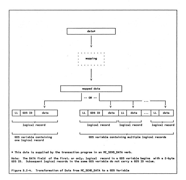
single logical record. MC\_MAX\_SEND\_SIZE is used only to determine how many logical records to create from the data; it is not used to determine whether enough data exists to be sent to the partner LU. (See Figure 5.2-4.)
