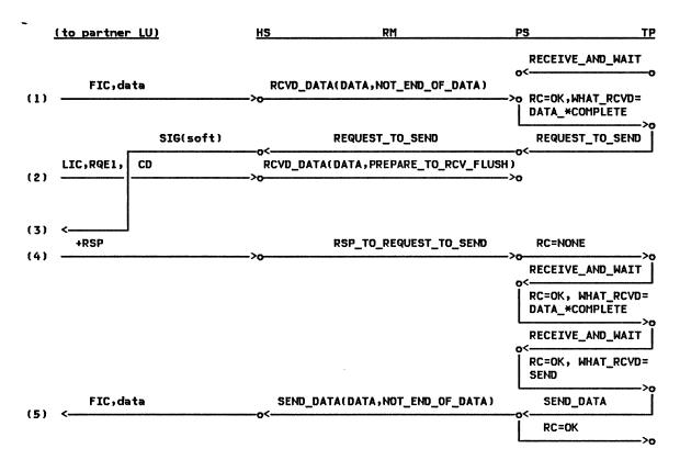
Figure 2-110. REQUEST\_TO\_SEND, Received in Receive State --Local LU
