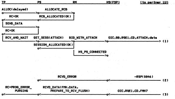
Figure 2-41. ALLOCATE (delayed), RECEIVE\_AND\_WAIT (by First Speaker) --Local LU
