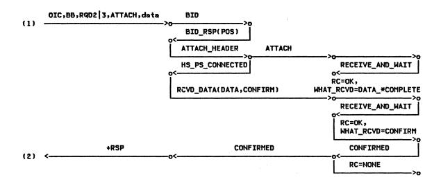
Figure 2-46. ALLOCATE (delayed), CONFIRM (by Bidder) -- Remote LU
