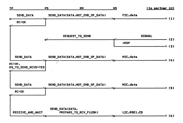
Figure 2-107. REQUEST\_TO\_SEND, Received in Send State --Remote LU
