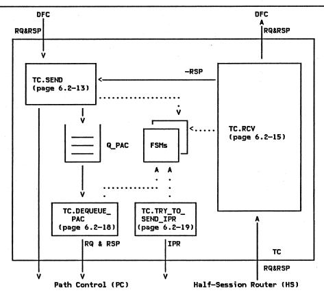
Figure 6.2-3. Interrelation of TC.SEND and TC.RCV
