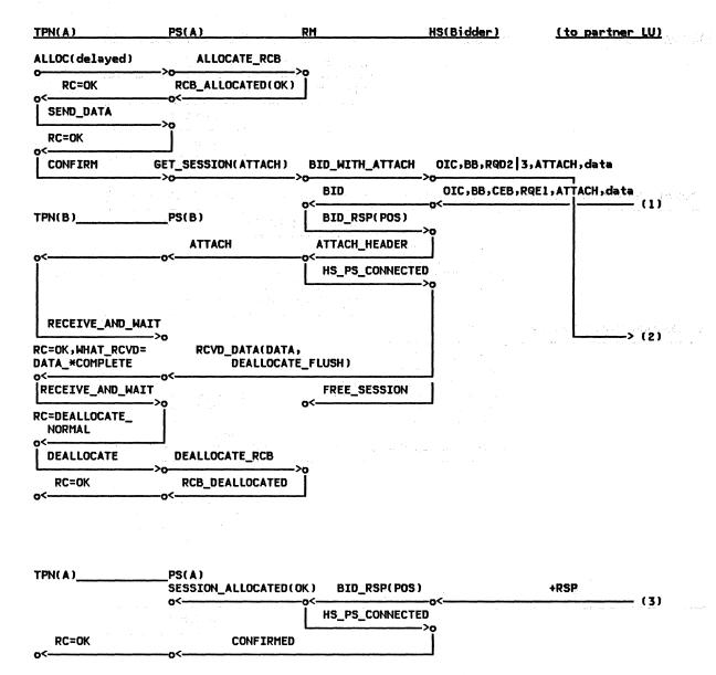
Figure 2-57. ALLOCATE (delayed) Race, Bracket Accepted --Bidder LU
