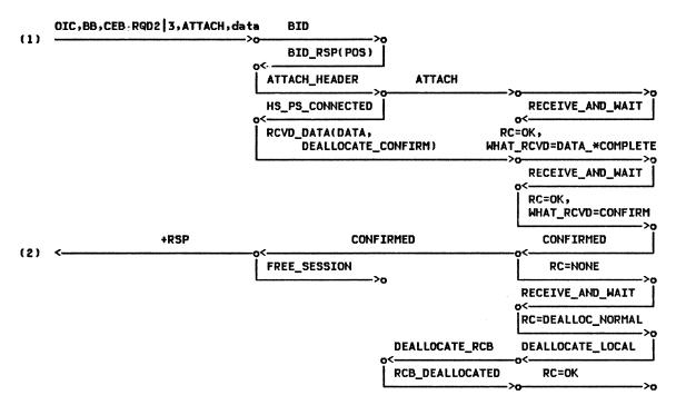
Figure 2-90. ALLOCATE (delayed), DEALLOCATE CONFIRM (by Bidder) -- Remote LU
