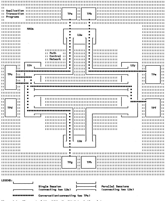
Figure 2-1. Placement of LUs within the SNA Network (Example)
