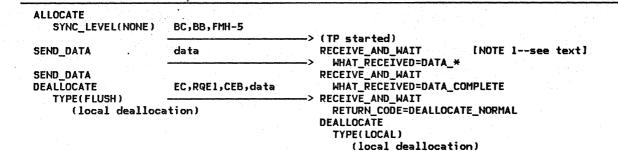
Figure 2-15. One-Way Conversation without Confirmation: Combines Sequences 1 and 3
