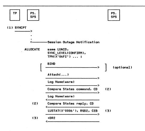
Figure 5.3-14. Resync After Conversation Failure
