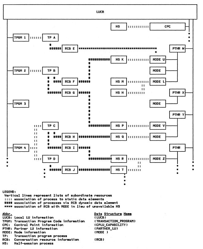
Figure 2-30. LU Dynamic Data Structures and Processes (Example)
