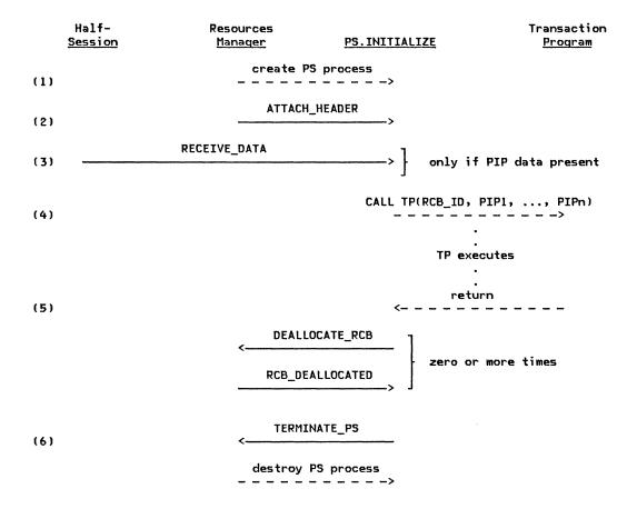
Figure 5.0-2. Initialization and Termination of Presentation Services and Transaction Program
