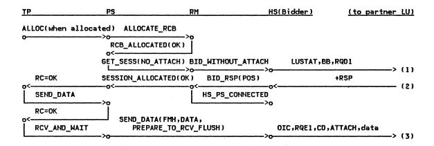
Figure 2-43. ALLOCATE (when allocated), RECEIVE\_AND\_WAIT (by Bidder) -- Local LU
