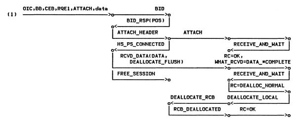
Figure 2-82. ALLOCATE (delayed), DEALLOCATE FLUSH (by First Speaker) -- Remote LU
