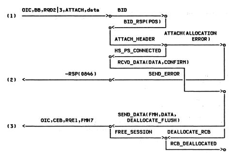
Figure 2-50. ALLOCATE (delayed), CONFIRM (by Bidder), Attach Error --Remote LU
