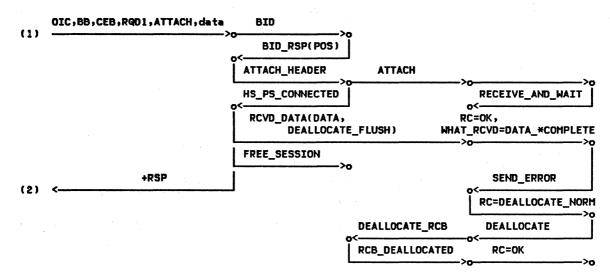
Figure 2-88. ALLOCATE (delayed), DEALLOCATE FLUSH (by Bidder) to SEND\_ERROR --Remote LU
