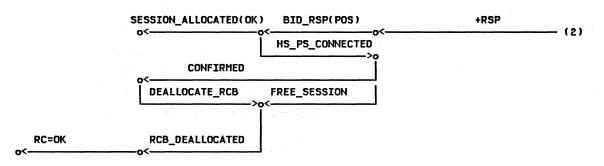
Figure 2-89. ALLOCATE (delayed), DEALLOCATE CONFIRM (by Bidder) --Local LU
