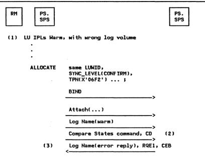
Figure 5.3-17. Log Name Mismatch during Resync
