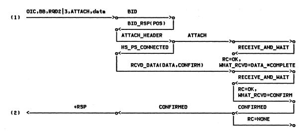
Figure 2-38. ALLOCATE (when allocated), CONFIRM (by First Speaker) -- Remote LU
