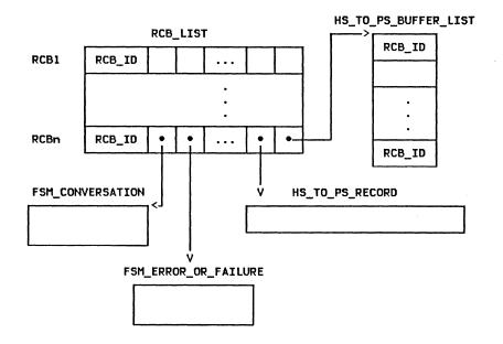
Figure 5.1-4. Resource Control Block (RCB)
