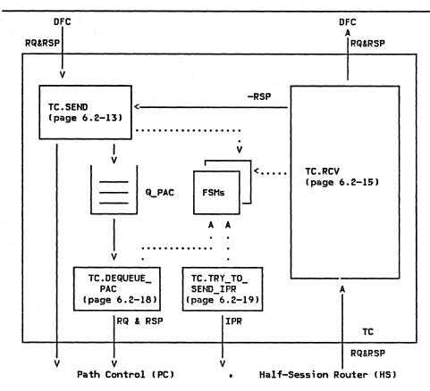
Figure 6.2-3. Interrelation of TC.SEND and TC.RCV
