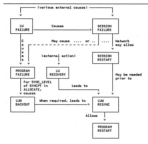
Figure 5.3-1. Relationships among Failures and Recovery
