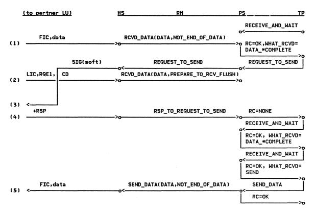
Figure 2-113. REQUEST\_TO\_SEND, Received in Receive State --Local LU
