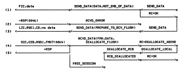
Figure 2-79. DEALLOCATE ABEND Issued in RCV, Between-Chain State -- Remote LU
