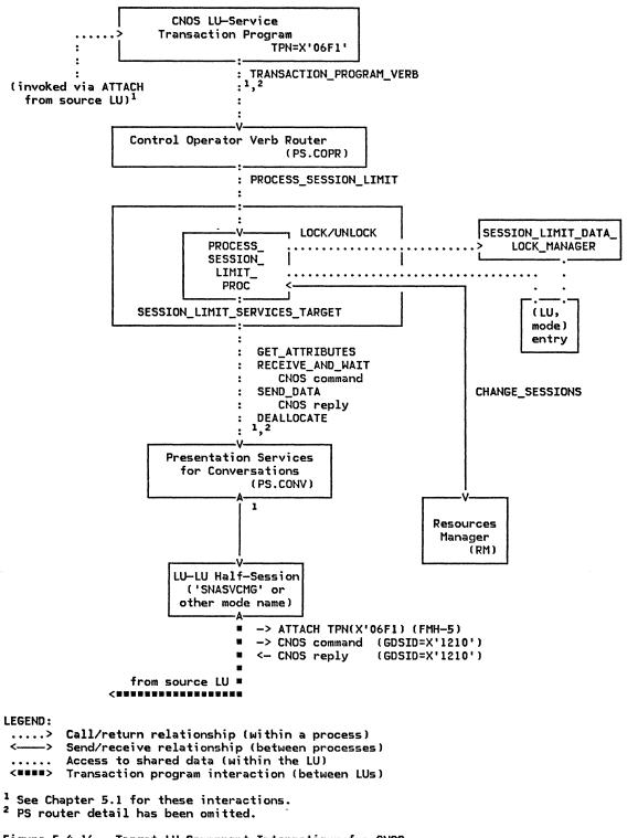
Figure 5.4-16. Target-LU Component Interactions for CNOS
