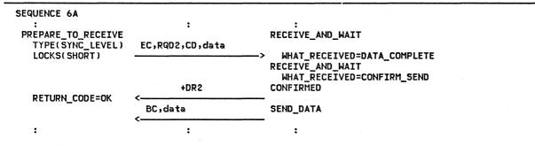
Figure 2-12. Conversation Turnaround with Confirmation, using LOCKS(SHORT):
