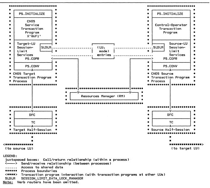
Figure 5.4-5. CNOS Process Interactions at a Single LU
