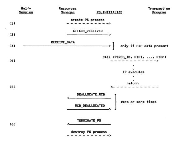
Figure 5.0-2. Initialization and Termination of Presentation Services and Transaction Program
