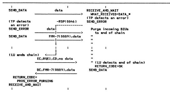
Figure 2-21. SEND\_ERROR Issued by both Sender and Receiver (SEND\_ERROR Race):
