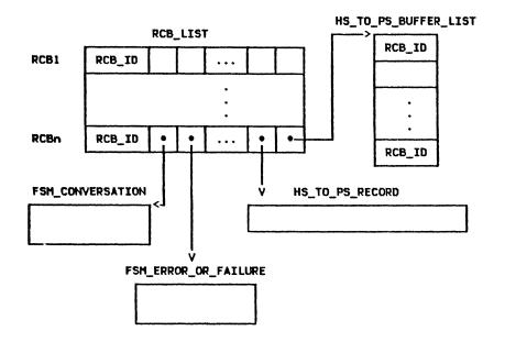
Figure 5.1-4. Resource Control Block (RCB)
