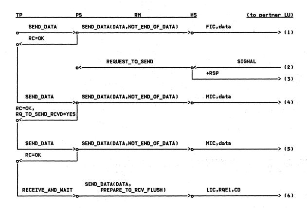
Figure 2-110. REQUEST\_TO\_SEND, Received in Send State -- Remote LU
