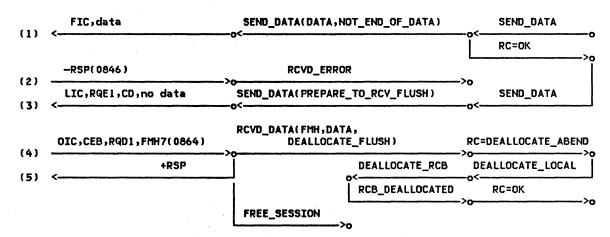
Figure 2-81. DEALLOCATE ABEND Issued in RCV, In-Chain State -- Remote LU
