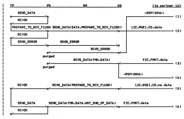
Figure 2-104. SEND\_ERROR Crossing SEND\_ERROR, Both Issued in Receive State --Remote LU
