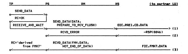
Figure 2-108. SEND\_ERROR at End-of-Chain --Remote LU
