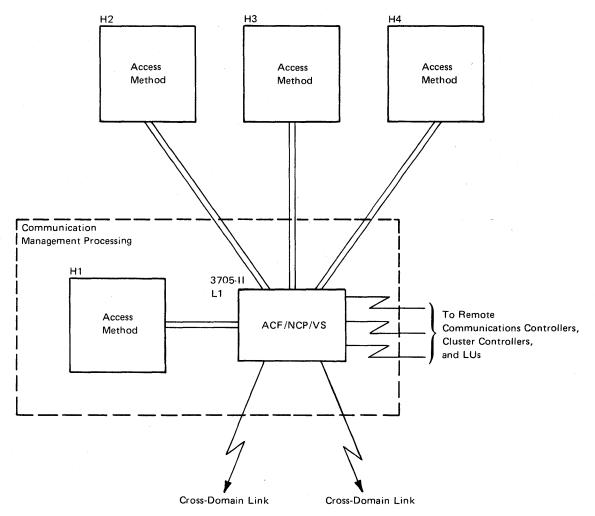
Figure 3-13. Possible Implementation of a Communication Management Configuration
