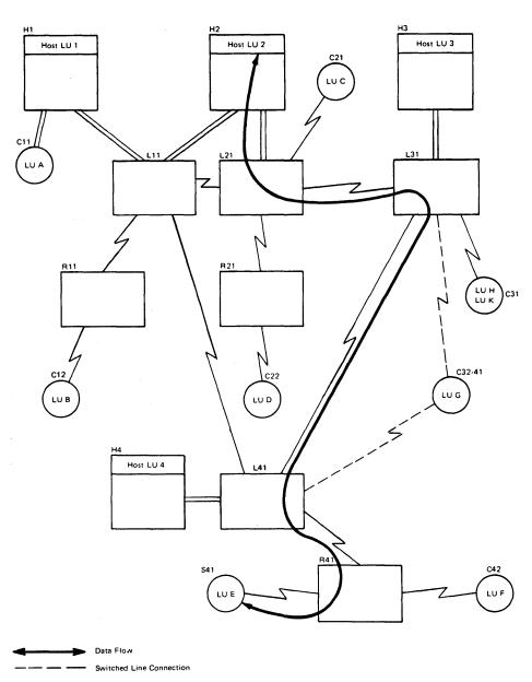
Figure 3-11. Data Flow Through an Intervening Domain
