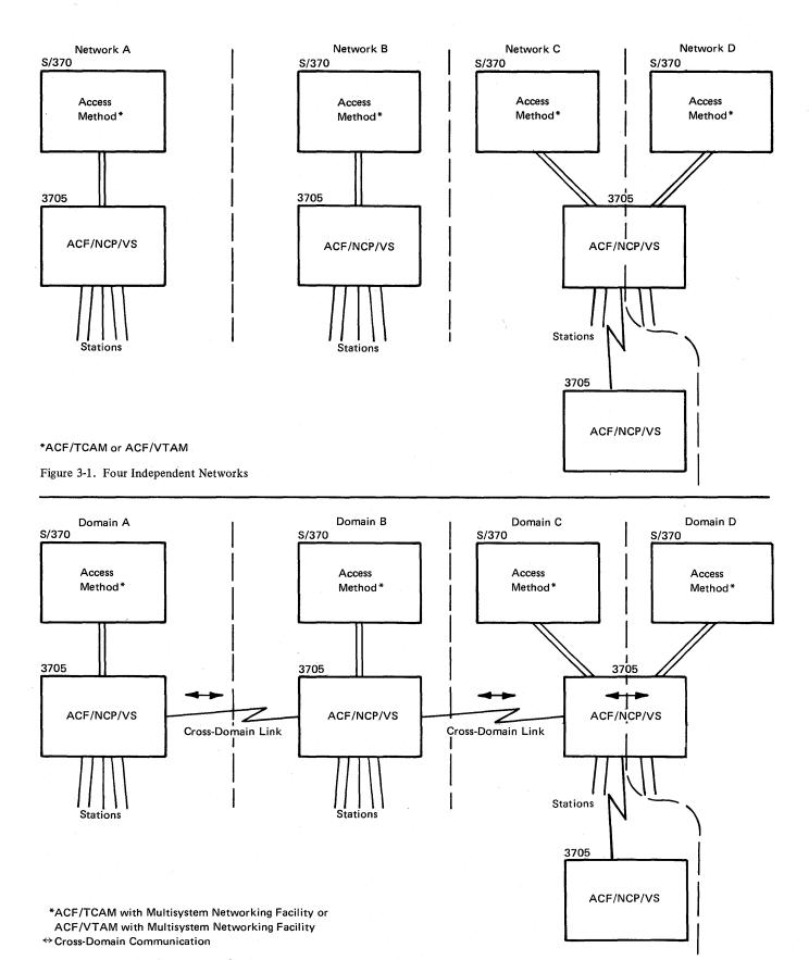
Figure 3-2. Four Networks Consolidated into a Single, Four-Domain Network
