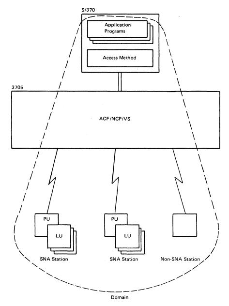
Figure 2-2. A Single-Domain Network Configuration
