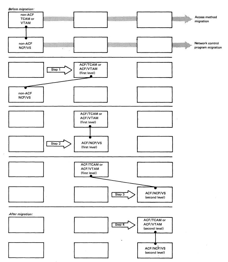
Figure 2-5. Step-by-Step Access Method/Network Control Program Migration
