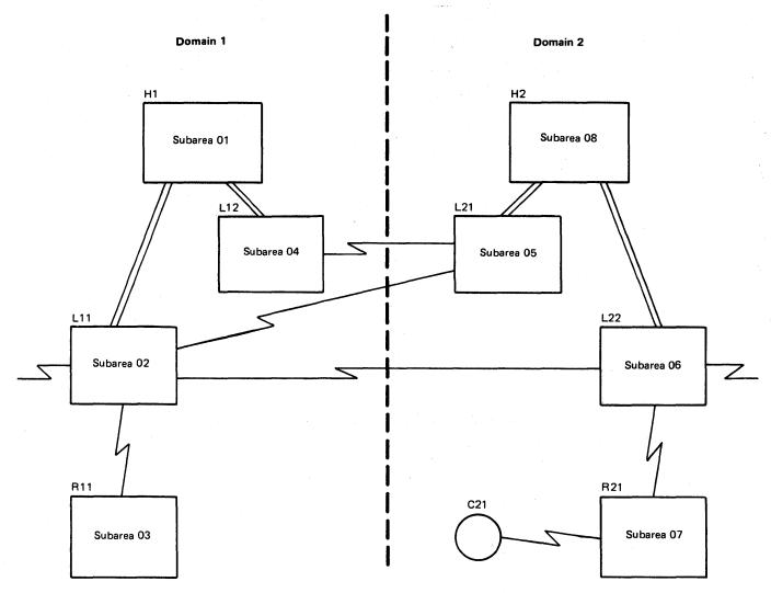
Figure 3-6. Configuration Having Multiple Paths Between Domains
