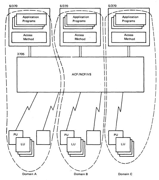
Figure 2-3. A Configuration of Multiple Single-Domain Networks
