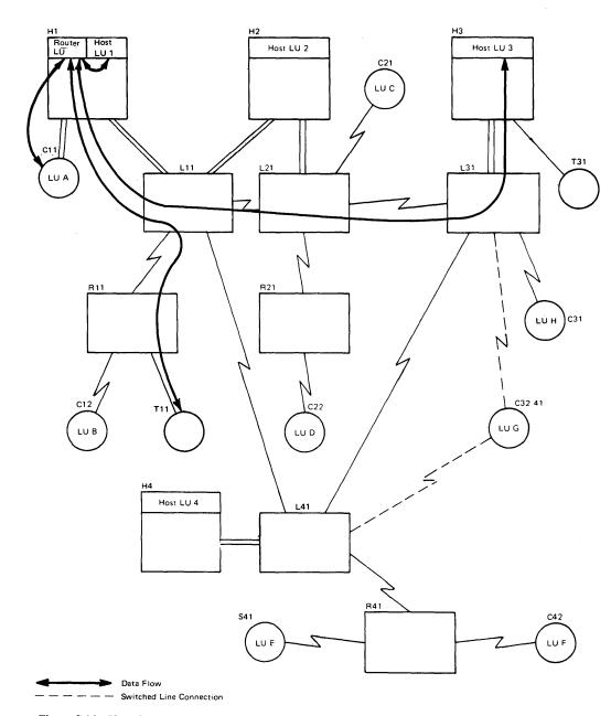
Figure 3-12. Use of a Router or Message Handler
