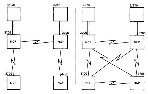
Figure 4-1. Links between NCPs Supported by ACF Level 2
