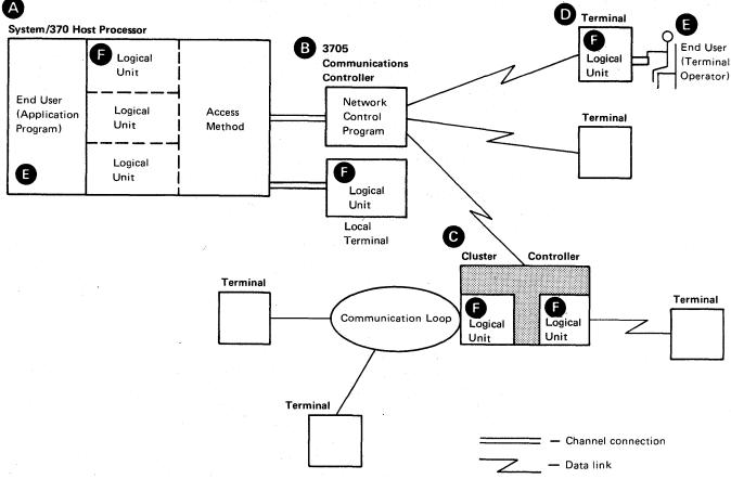
Figure 2-1. Elements of an SNA-Based Data Communication Network
