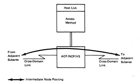
Figure 3-7. Intermediate Node Routing by ACF/NCP/VS
