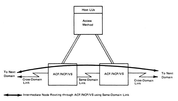
Figure 3-8. Intermediate Node Routing Between Local Communications Controllers in the Same Domain
