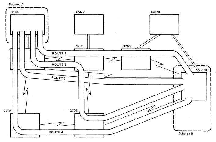
Figure 4-5. Two Subareas Joined by Four Routes
