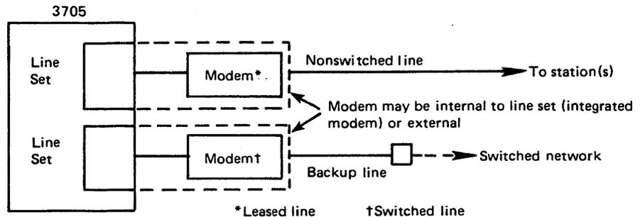
The principal and backup lines are represented to the NCP by separate LINE macros. The modem (3872, 3874, or 3875) at the remote station must be equipped with the switched network backup feature (or a separate switched network modem provided in addition to the regular modem, with provision for switching the station from one to the other).
