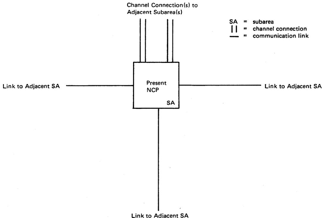
Figure 1-1. Network Control Program and Links to Adjacent Subareas
