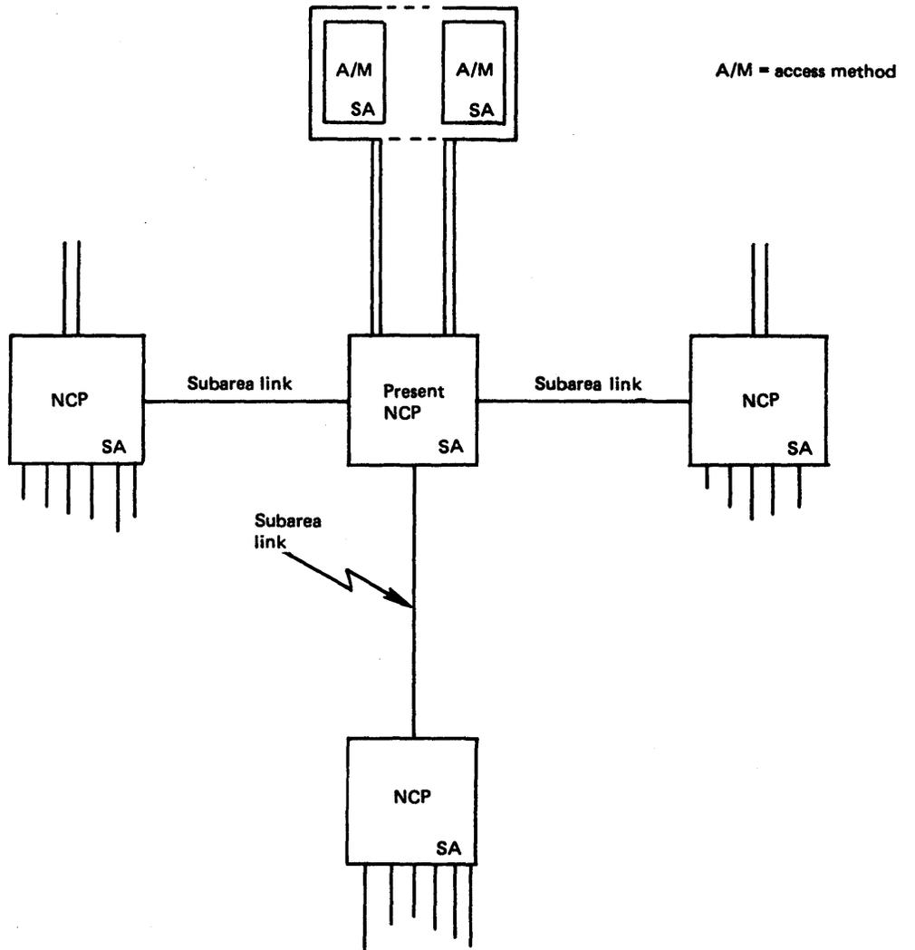
Figure 1-2. Relationship of Network Control Program to Adjacent Subareas
