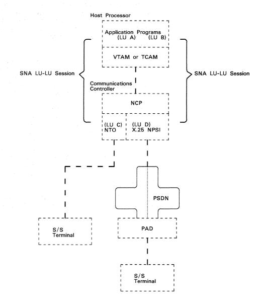
Figure 2-3. Configuration of NCP Containing Both the X.25 NCP Packet Switching Interface and NTO
