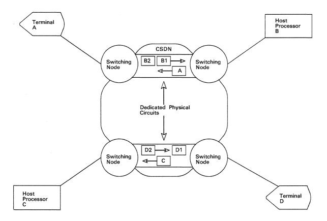
Figure 1-1. Circuit-Switched Data Network (CSDN)
