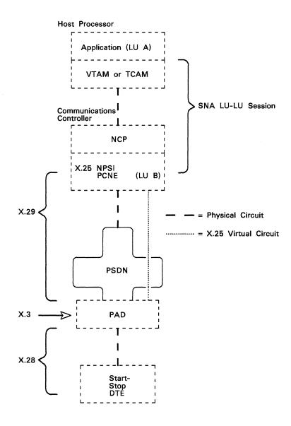
Figure 2-4. Host Processor Communicating with an X.28 Start-Stop DTE Using the Integrated PAD Function
