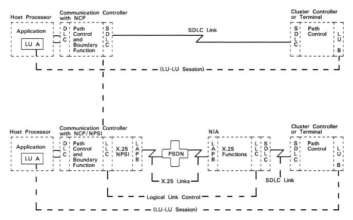
Figure 1-6. SNA-to-SNA Configuration Comparing SDLC Links to Packet Switching
