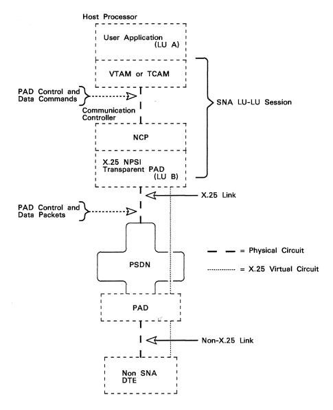
Figure 2-5. Host Processor Communicating with a Non-SNA DTE Using the Transparent PAD function
