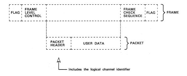
Figure 1-4. Frame and Packet
