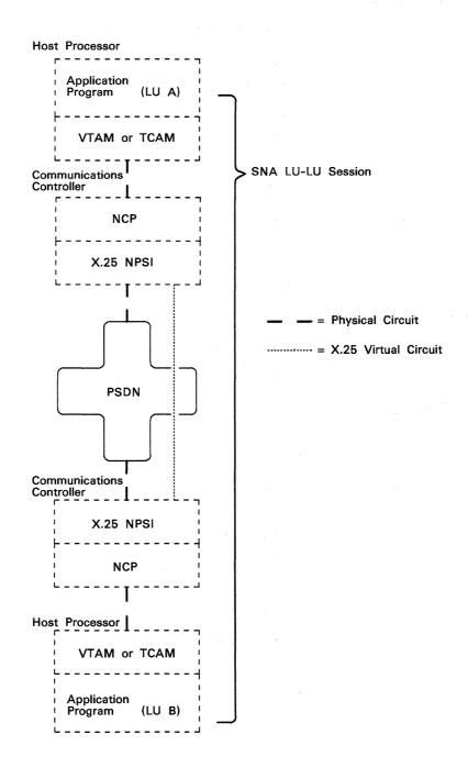
Figure 2-8. Host-to-Host Connection Using the X.25 NCP Packet Switching Interface
