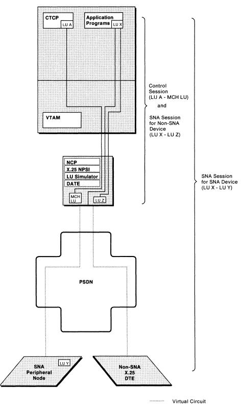
Figure 15. SNA Host Node to SNA Peripheral Node or to Non-SNA X.25 DTE (DATE)
