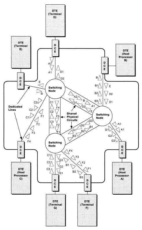
Figure 3. Packet Switched Data Network (PSDN)
