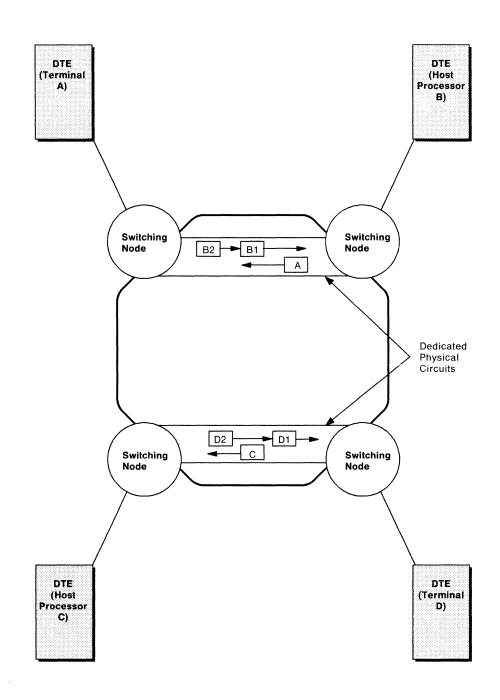
Figure 2. Circuit Switched Data Network (CSDN)
