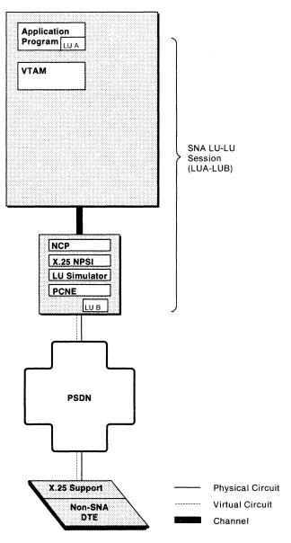
Figure 11. SNA Host Node to Non-SNA X.25 DTE (PCNE)
