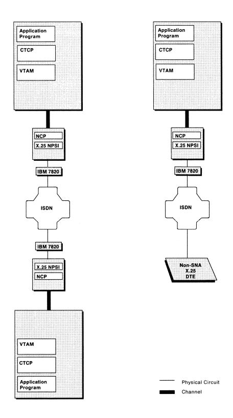
Figure 16. SNA Host to ISDN (X.21 Switched Connection)
