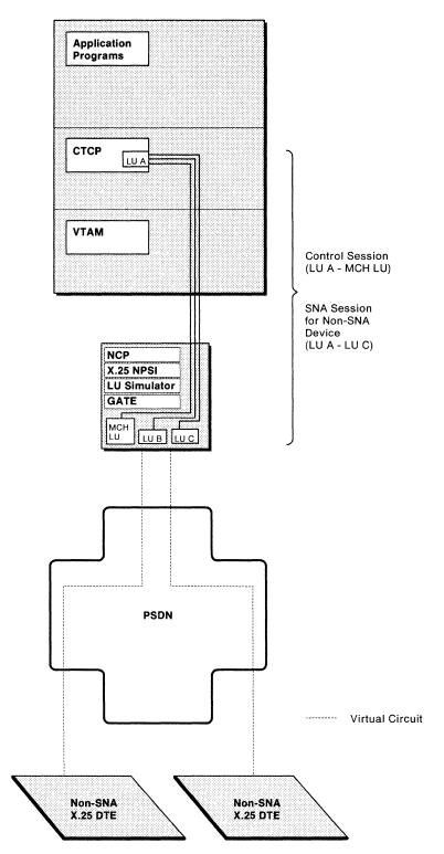
Figure 14. Host Node to Non-SNA X.25 DTE (GATE)
