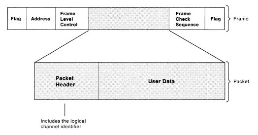
Figure 5. Frame and Packet
