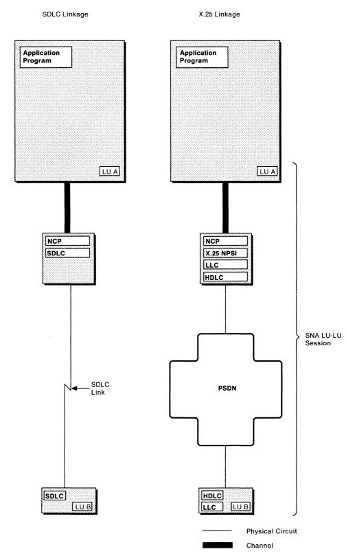
Figure 4. Comparison of SDLC and X.25 Linkages in an SNA-to-SNA Configuration
