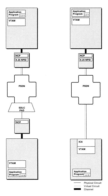
Figure 9. More Communication between Subarea Nodes
