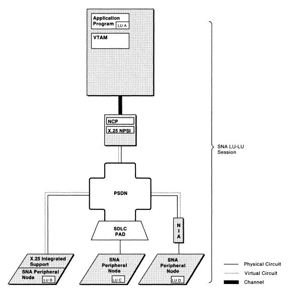
Figure 10. SNA Host Node to SNA Peripheral Node
