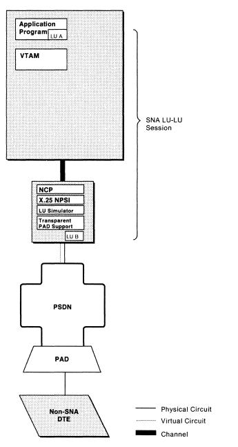
Figure 13. Host Node to Non-SNA X.25 DTE (Transparent PAD Support)
