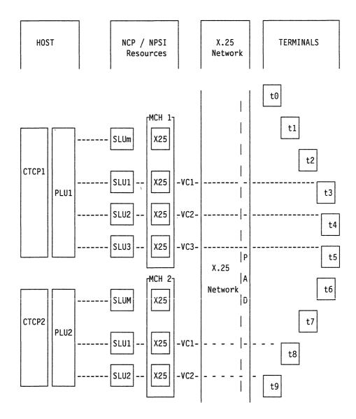
Figure 13. Fast Connect with One CTCP for One Physical Circuit
