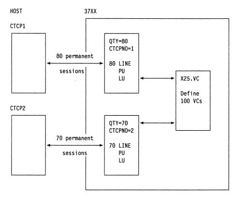
Figure 14. Fast Connect with Two CTCPs for One Physical Circuit
