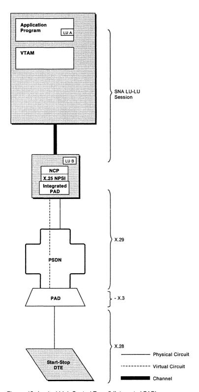
Figure 15. Logical Link Control Type 5 (Integrated PAD)
