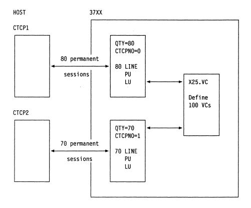
Figure 19. Fast Connect with Two CTCPs for One Physical Circuit
