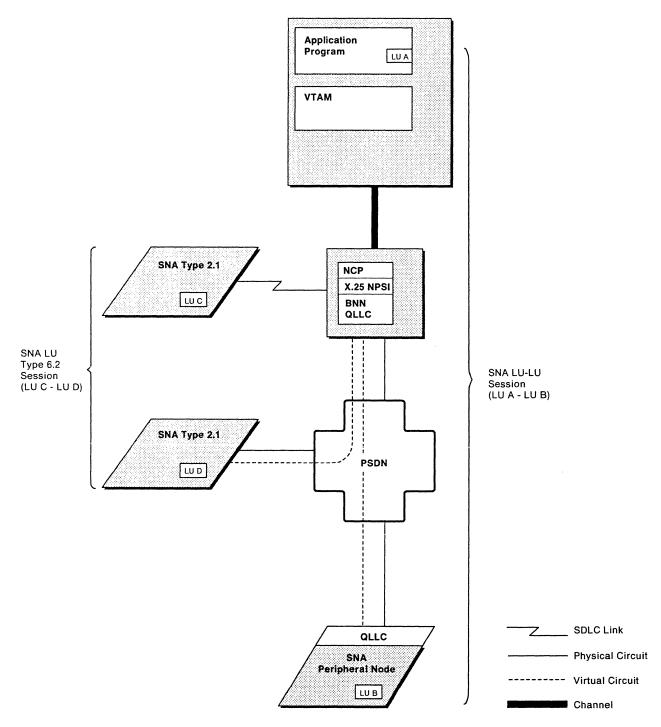
Figure 7. Logical Link Control Type 3 (Peripheral Node)
