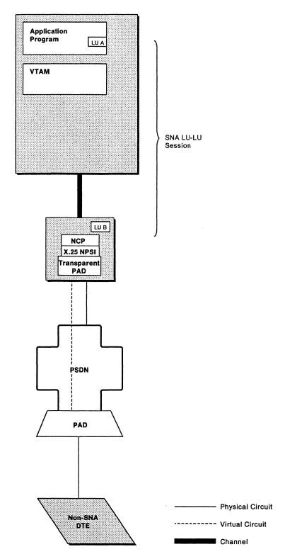
Figure 16. Logical Link Control Type 5 (Transparent PAD)
