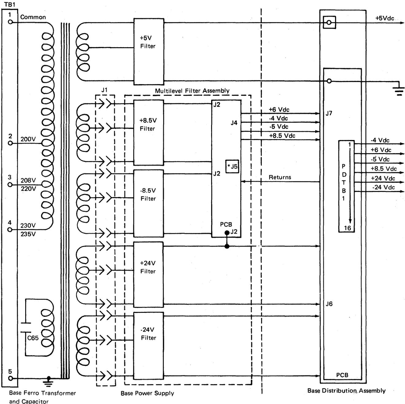
\* J5 is used to send an overcurrent sense signal to the C-A1 board
