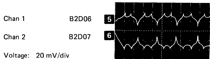
Chan 1 B2D06 5 Chan 2 B2D07 6 Voltage: 20 mV/div Time: 1 \mu s/div Trigger: External + D2P11, Chopped AC Input
