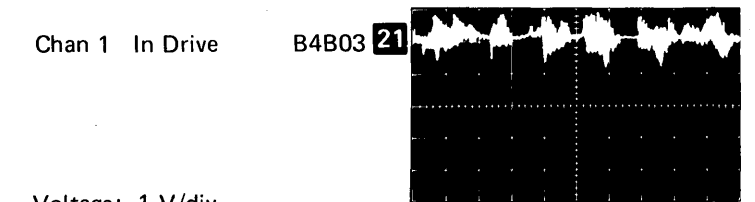
Chan 1 In Drive B4B03 21 Voltage: 1 V/div Time: 1 ms/div Trigger: External + C4J13 - Speed Transducer
