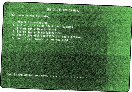
The End of Job Option Menu is used to specify what you want done with the work you have just completed. You can, for example, return to what you were doing, or end the job and get a printed listing of the statements in the source or procedure member. Select the appropriate end of job option and press the Enter key; the SEU End of Job display appears.
