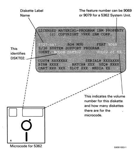
For a 5362 System Unit, there are three microcode diskettes. For the release update, use the diskette labeled DSKT02.
