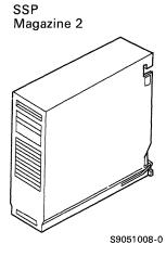
2c. Insert the SSP diskettes (labeled 5727-SS1) into the diskette magazines. Put the first SSP diskette (VOL01) in slot 1 of the magazine labeled SSP Magazine 1. Put the second SSP diskette (VOL02) in slot 2, and so on until the first ten SSP diskettes are in SSP Magazine 1.
