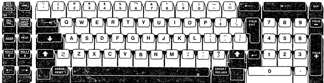
Figure 3-24. 5251 Typewriterlike Keyboard
