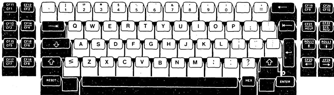
Figure 3-5. System Console Keyboard
