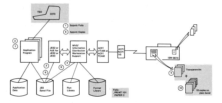
Figure 7. Preparing a Presentation Using TSO, the IBM 6670, and the MVS/Information Distribution Workstation Support Program
