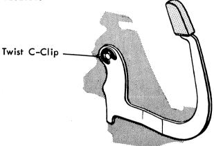
Excessive play of release levers in typewriters prior to this change can be reduced by applying a slight twist to the C-Clip, being careful not to create a bind in the levers.
