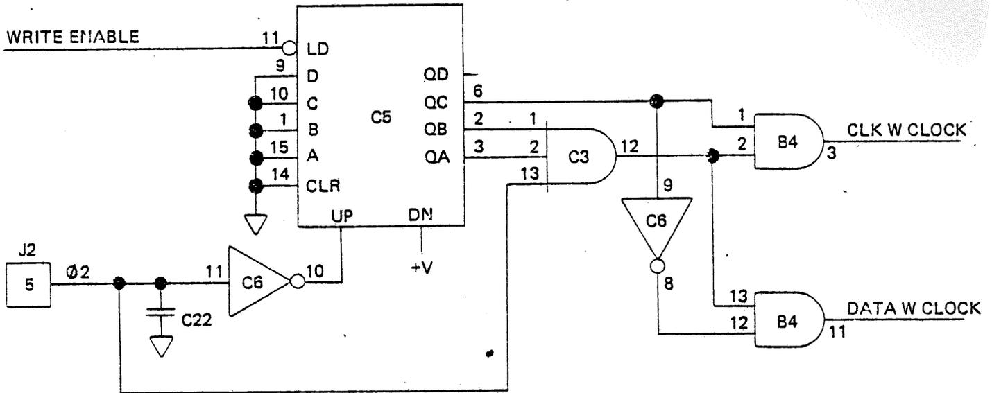
FIGURE 10 Clock W Clock/Data W Clock Generation
