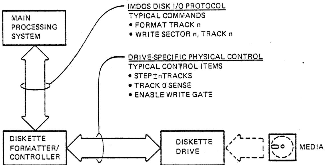
FIGURE 1 Disk System, Functional Block Diagram
