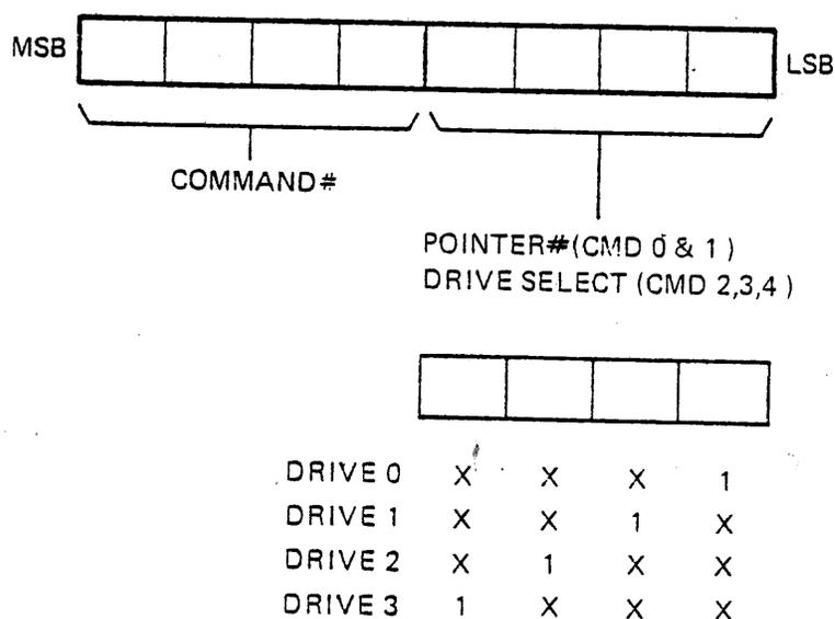
FIGURE 15 Byte Command Format
