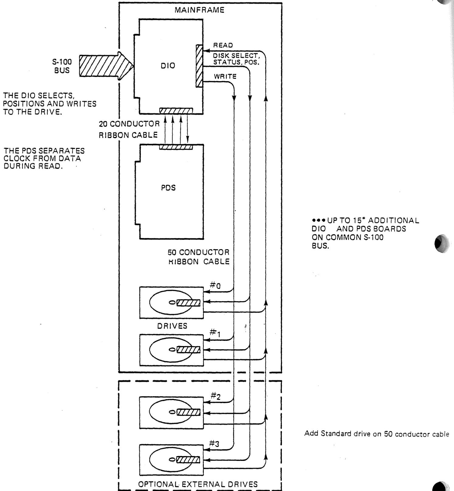
FIGURE 2 DIO/PDS Block Diagram
