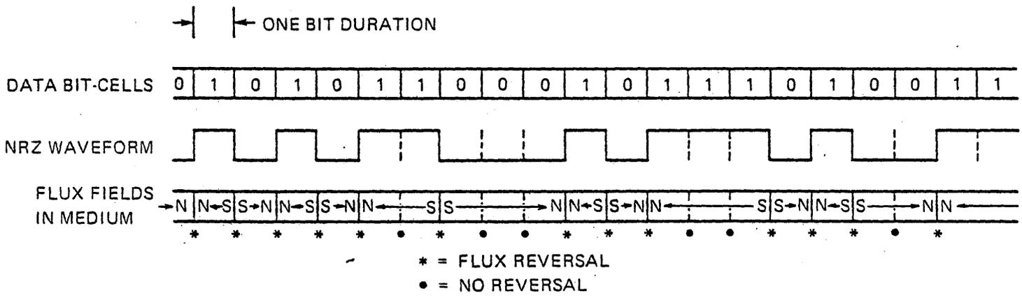
FIGURE 6 Bit-Cells and Flux Reversals
