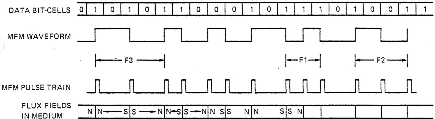
FIGURE 8 MFM Data Encodation
