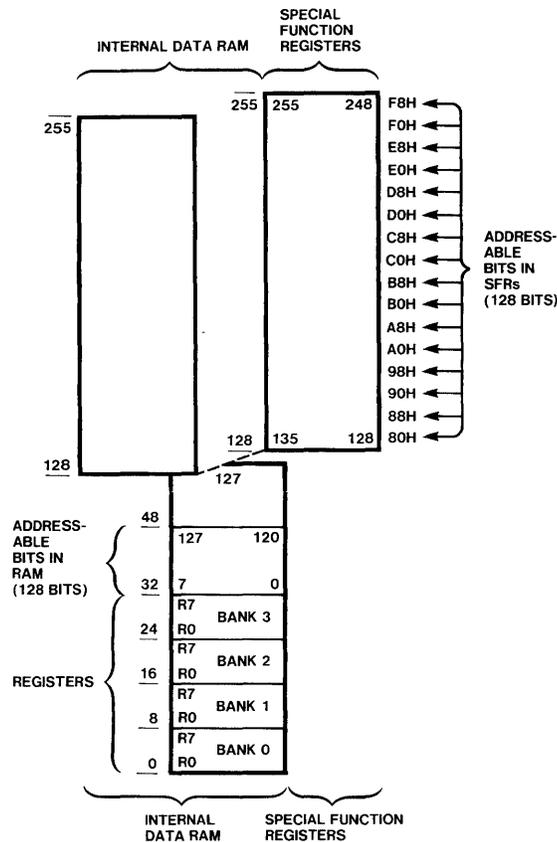
Figure 3-2. Internal Data Addressing Modes
