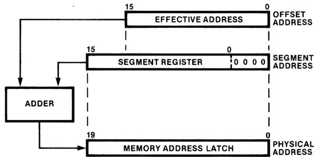
The 8086 memory can be thought of as an arbitrary number of segments. A byte or word within a segment is addressed with a 16-bit offset address. The 8086 automatically adds the offset address to the shifted 16-bit segment address, creating a 20-bit physical address.
