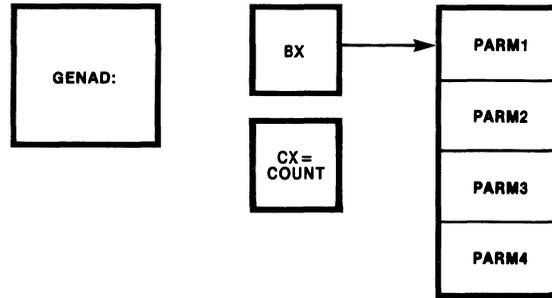
Example 4 below shows how this process can be written in the 8086 assembly language. GENAD returns the sum in the accumulator. It receives the address of the array in the BX register, and the number of array elements in CX.
