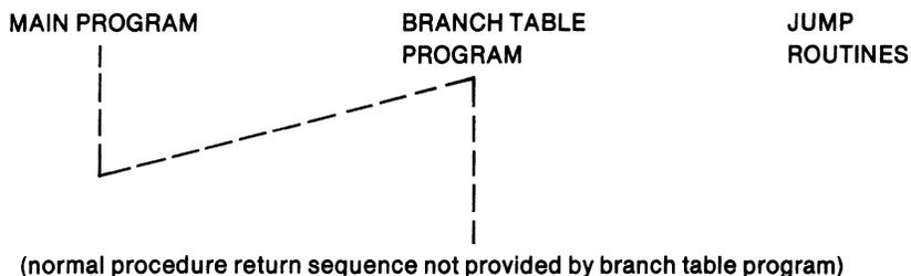
Example 1 below is a routine which transfers control to one of the eight possible procedures depending on which bit of the accumulator is 1.
