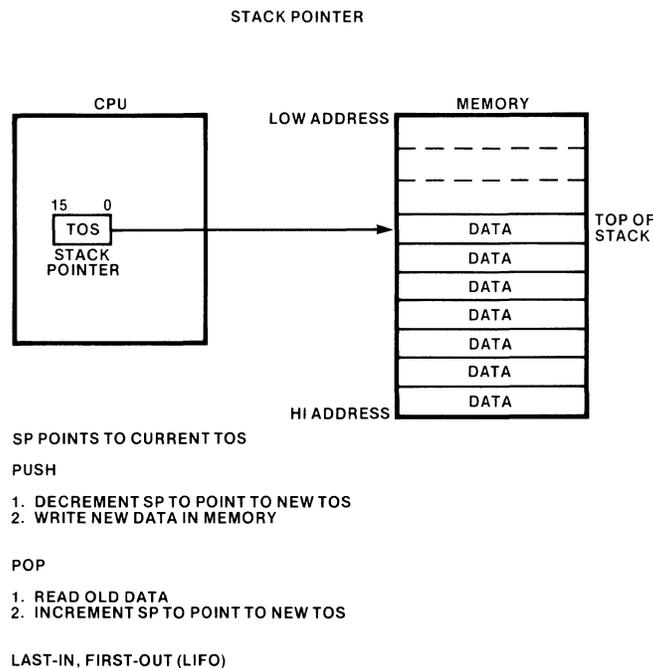
"Stack" is a most descriptive term because you can always put something on top of the stack, like a dish stacker. You can PUSH a new dish (word) on top, or POP the last one on top off into a destination you specify. In terms of programming, a procedure can call a procedure, and so on. The only limitations to the number of items that can be added to the stack are the amount of RAM available and the 64K limit on segments.
