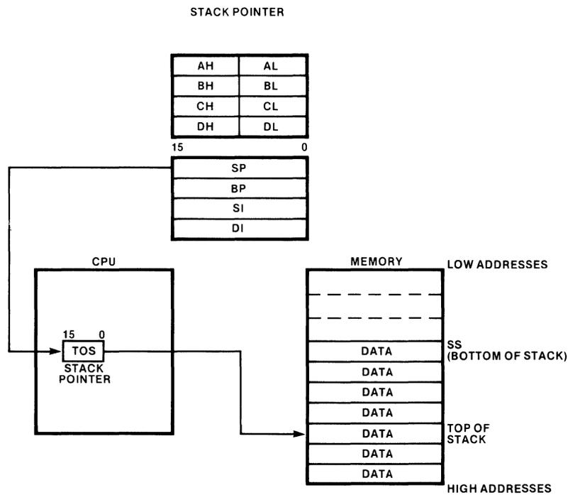
The stack is also used for temporary storage of parameters for use in such a procedure. Before the `CALL`, the calling routine can first `PUSH` the data onto the stack. The called routine can then simply access the stack directly. Though this has certain advantages, it leaves the data sitting on the stack, violating the normal expectation that the `RETURN` will leave the stack as it was before the calling program used it. In this situation the called routine can end with the statement:
