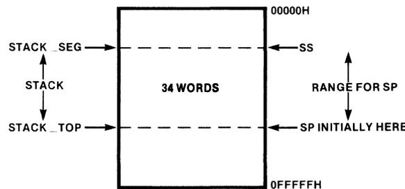
Note that the length of the combined segment is 34 words, the sum of the lengths of the pieces; but that the top-of-stack variables “stack\_top” and “top\_stack”, whose names are local to each module, are assigned the same offset (68D = 44H bytes) at the high end of memory. You can set the stack segment base and the stack pointer by the instructions (in module 1):
