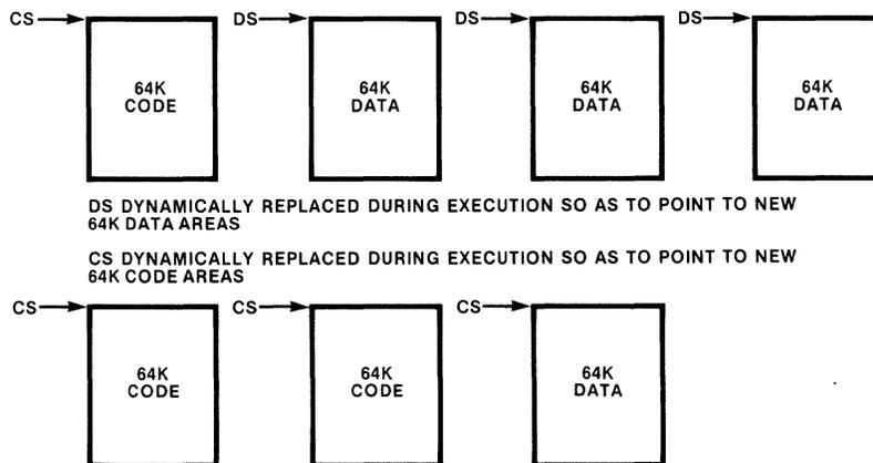
In order for the automatic addressing described above (under Memory Addressing) to occur properly, you must load the segment registers with the paragraph numbers, i.e., the segment base-addresses, that you want used for each section of code. You do this by using the name of your segment, e.g.,
