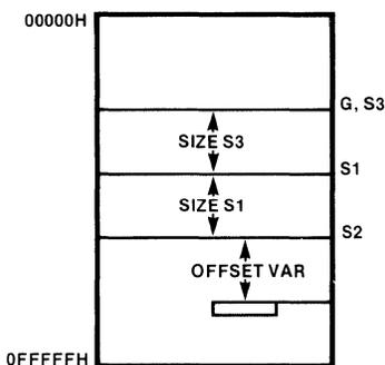
The value of `OFFSET G:VAR` will include the sum of the size of `S3`, the size of `S1`, and `OFFSET S2:VAR`, but this sum must be adjusted for the align-types and ending points of `S3`, `S2`, and `S1`.
