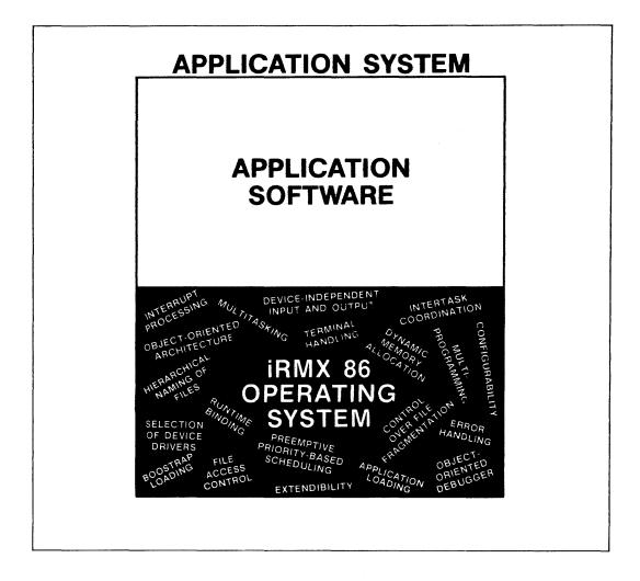
Figure 4-1. Features of the iRMX 86<sup>TM</sup> Operating System
