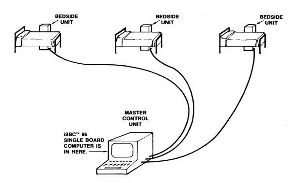
Figure 5-1. The hardware of the dialysis application system
