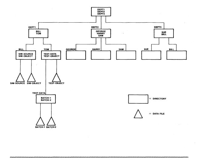
Figure 5-1. Example of a Named-File Tree
