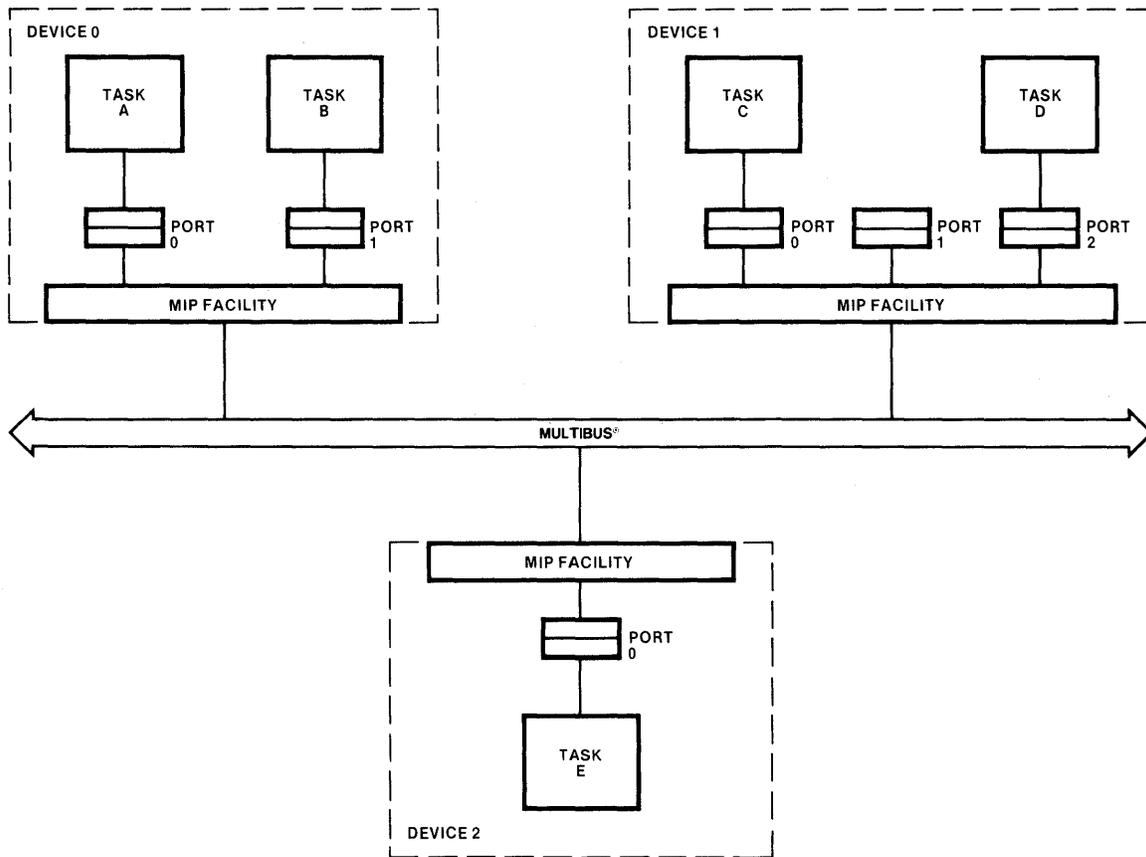
Figure E-2. A Configuration of Ports
