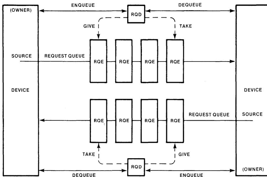
Figure E-5. Conceptual Structure of a Channel
