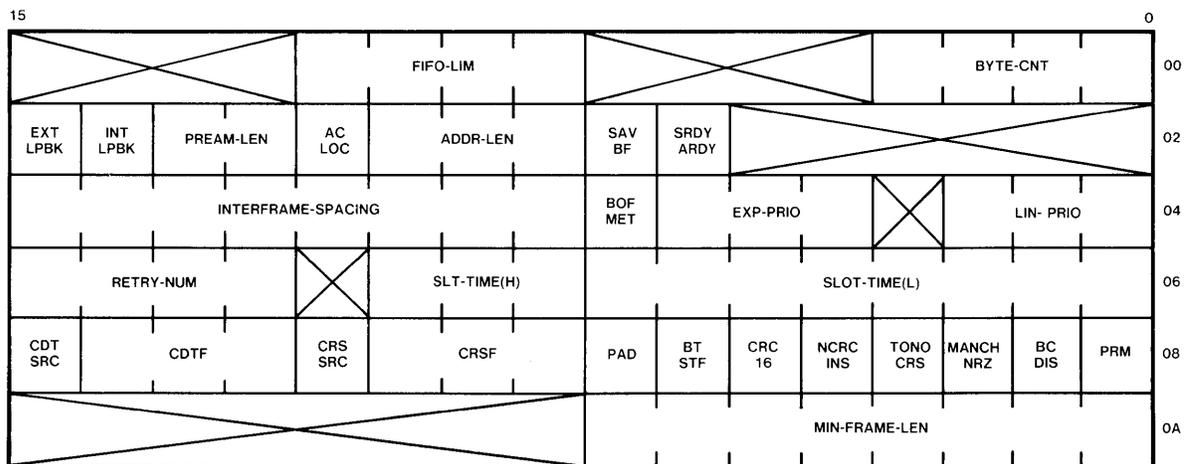
Figure D-1. CONFIGURE Command Argument Field
