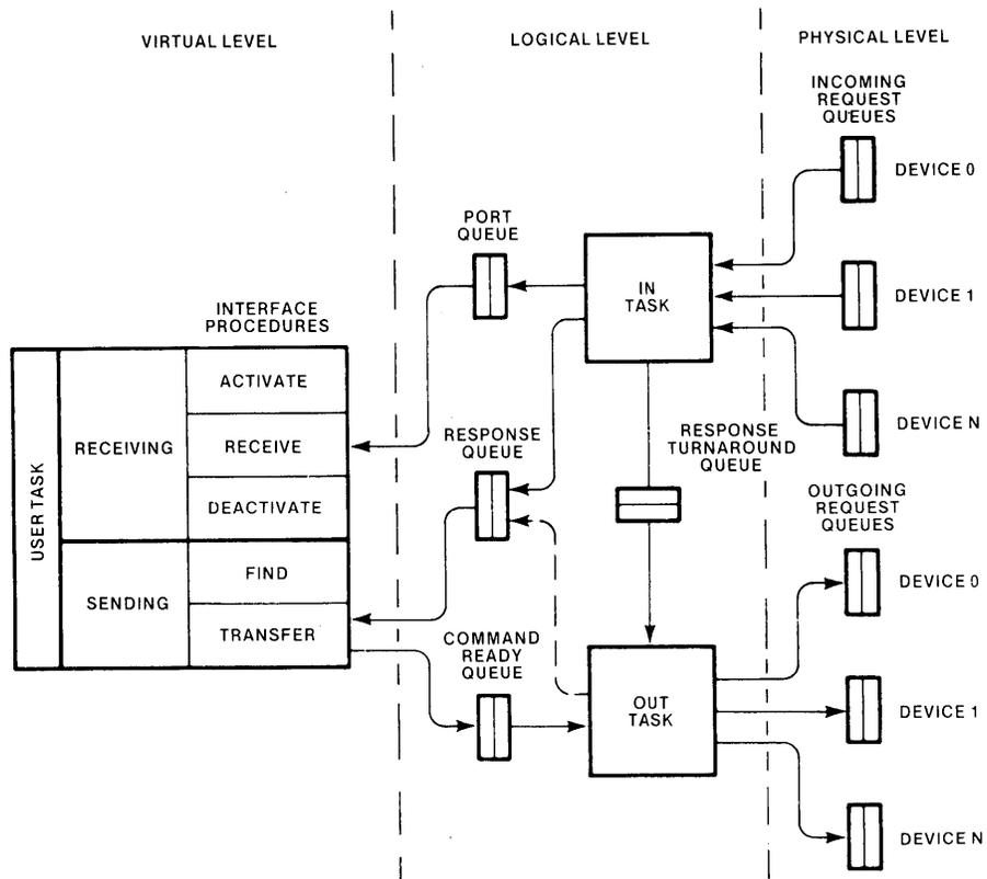
Figure E-3. Data-Flow Structure of the MIP Model
