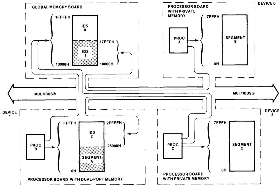
Figure E-6. Example of Interdevice Memory Segments
