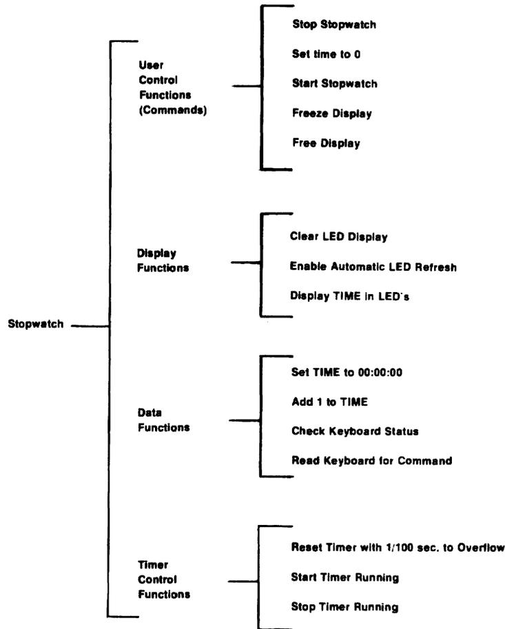
Figure C-1: Stopwatch Program Structure
