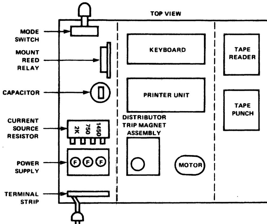
Figure 6-9. Teletypewriter Layout
