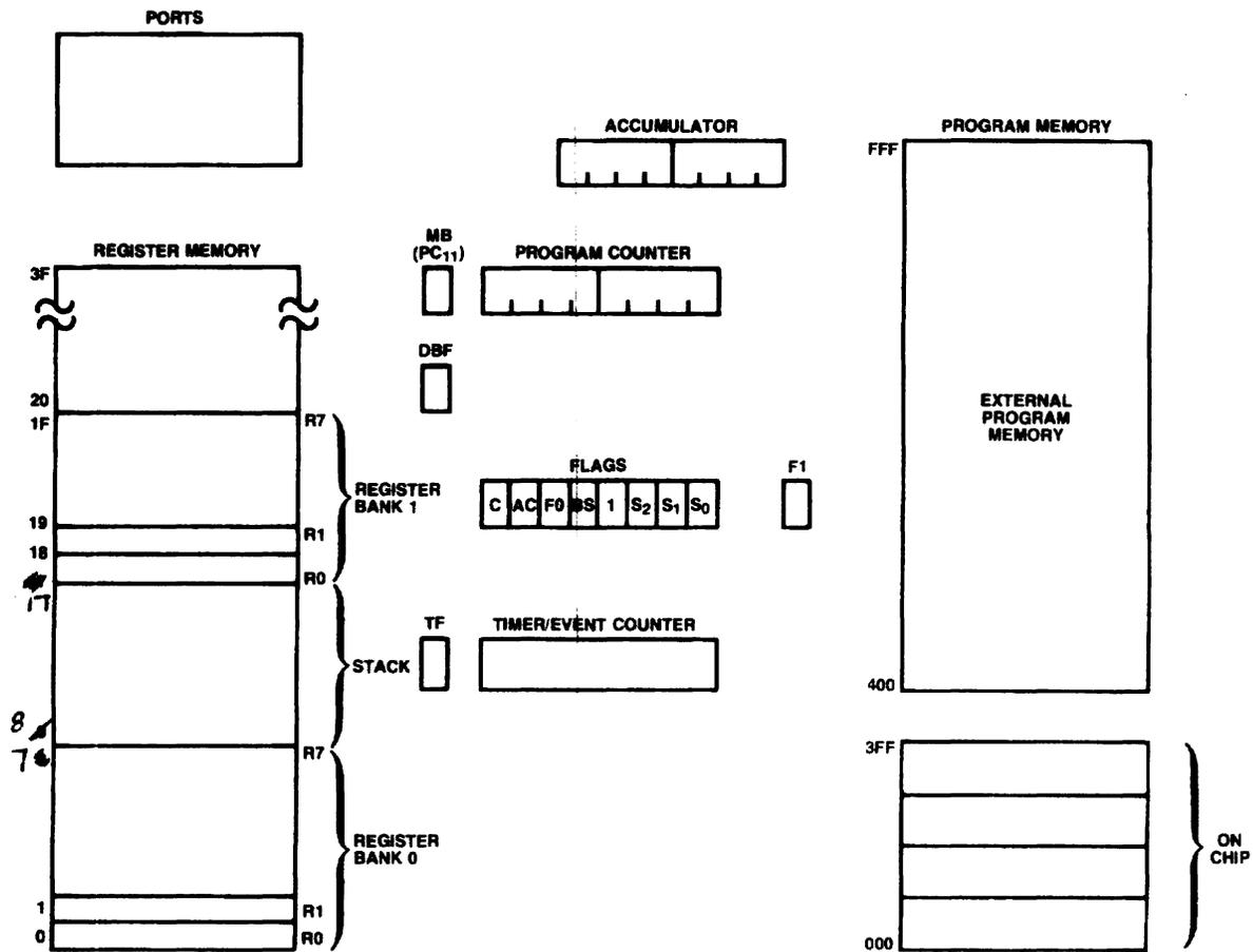
for completion. The MCS-48 computers have facilities which allow a program to be interrupted, made to perform more urgent tasks, and later be returned to the original activity through the use of a stack.
