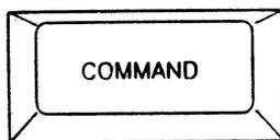
The Command Key is used in conjunction the alphanumeric keys to generate Escape sequences that may be assigned functions by the host program. The key is used by holding it down while striking another key. When operated by itself it generates no code.
