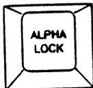
The Alpha Lock key, when engaged, makes all the alphabetic keys uppercase. It does not affect numeric and special character keys.
