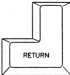
This key is used instead of the (Control M) combination to send the ASCII carriage return code <CR>.
