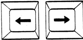
These keys generate codes that move the cursor in the direction of the arrows on the keys, one character cell per keystroke. When these keys are held down their codes are generated repeatedly.
