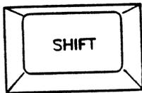
The two Shift keys are used interchangeably in conjunction with other keys to generate the uppercase ASCII codes. All the alphanumeric keys except for the Space Bar and DEL are affected by the Shift keys. The Shift keys are used by holding either of them down while operating another key. By themselves they generate no code.
