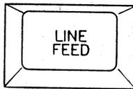
This key is used instead of the (Control J) combination to send the line feed code <LF>. When held down, it sends the code repeatedly.
