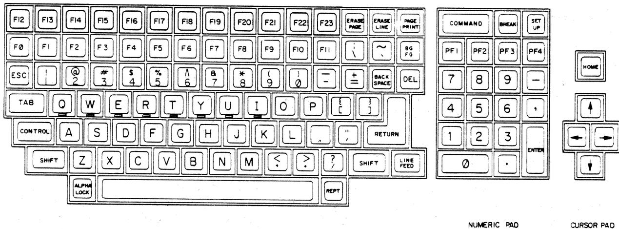
The keys grouped immediately to the left of the cursor pad are arranged in six rows. The top two rows contain special purpose keys whose special functions are discussed below. The bottom four rows constitute a numeric keypad similar to those found on standard office machines.
