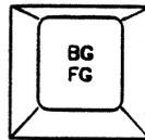
The FG/BG key is used to change the colors with which characters and plot blocks are displayed. Color change is accomplished by striking this key and then one of the following alphabetic keys: Q,W,E,R,T,Y,U,I (or, in some units, keys F0-F7). These keys represent the colors black, red, green, yellow, blue, magenta, cyan, and white respectively. Only characters displayed subsequently, beginning at the current cursor position are affected.
