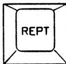
The Repeat key may be held down together with another key in order to transmit repeatedly the code or code sequence generated by that key.
