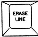
The Erase Line key is used to erase the contents of the display from the cursor position to the end of the line. It sends the following Erase Line (EL) command sequence: `<ESC>[0K`
