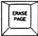
The Erase Page key is used to erase the display from the cursor position to the end of the page. The key generates the following Erase Display (ED) command sequence: `<ESC>[0J`
