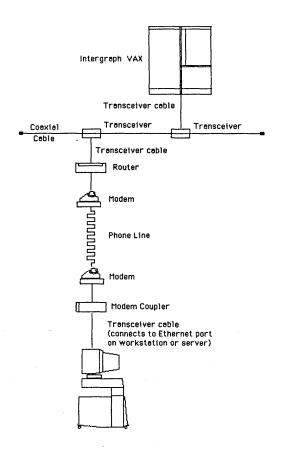
Figure 6-1. An Intergraph Workstation Connected to a Remote Ethernet Network
