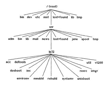
Figure 4-1. System V's Hierarchical Structure
