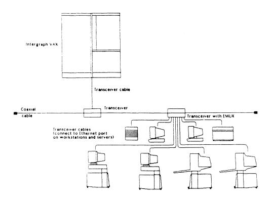
Figure 6-2. Intergraph Workstations and Servers Connected to an EMUX
