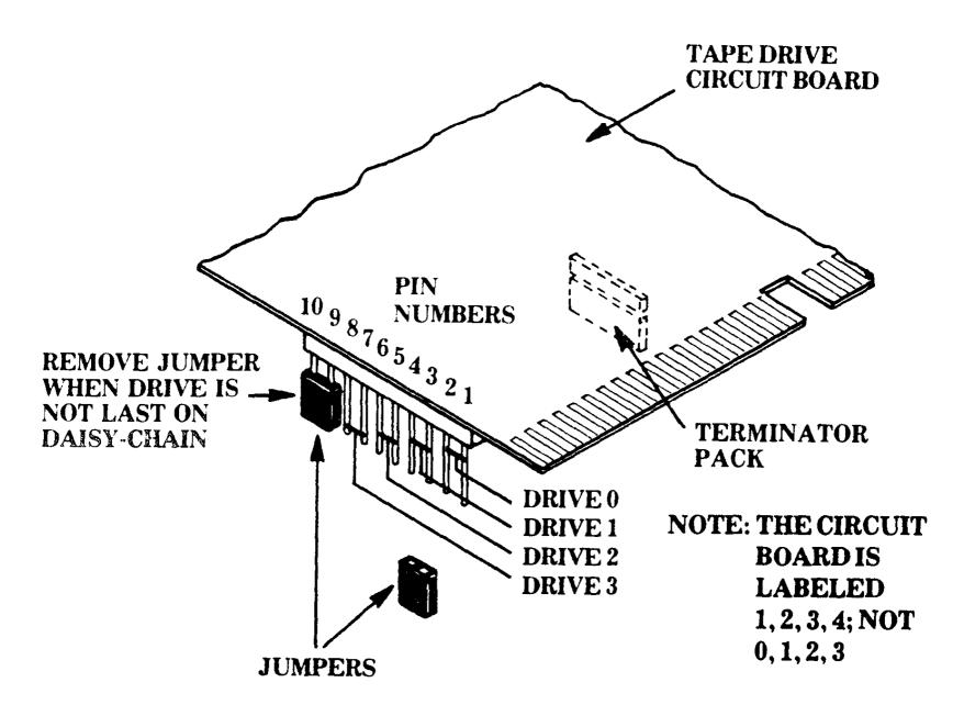
Figure B-1. Drive Assignment Jumpers
