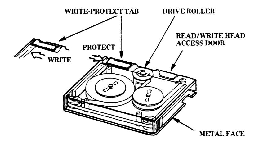
Figure 2-2. The Tape Cartridge
