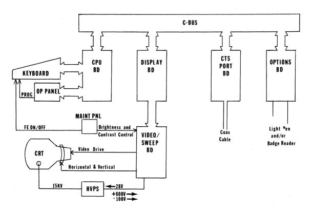
Figure 2.4 C270-III GENERAL BLOCK DIAGRAM
