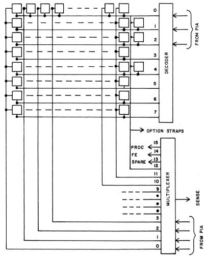
Figure 2.10 KEYSWITCH ADDRESSING TECHNIQUE
