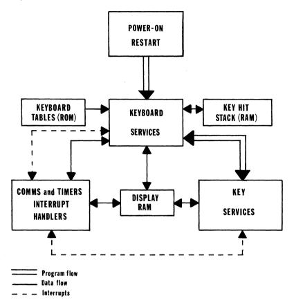
Figure 2.12 FIRMWARE BLOCK DIAGRAM
