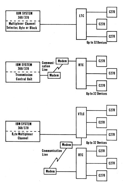
Figure 1.1 SYSTEM CONFIGURATOR
