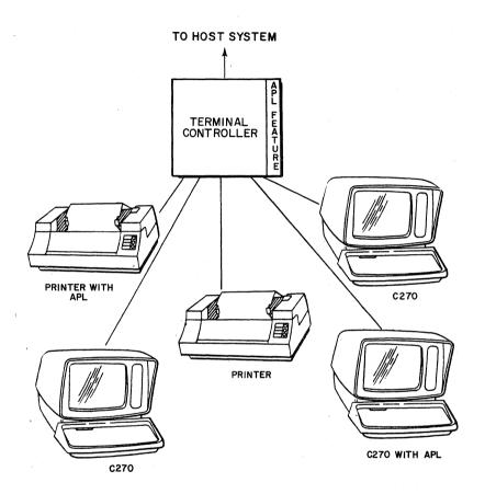
Figure B1.1 APL System Configuration
