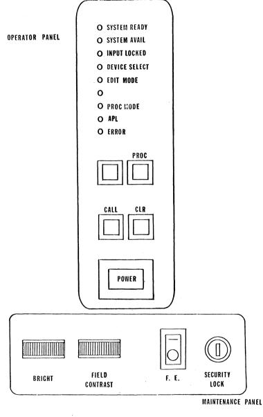
Figure B1.7 APL Operator Panels
