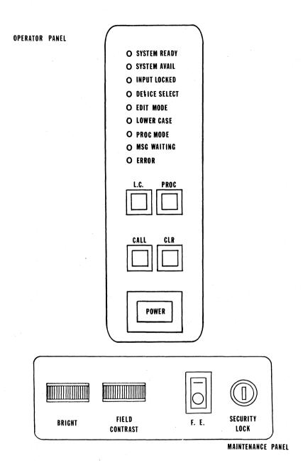
Figure 2.1 OPERATOR AND MAINTENANCE PANELS
