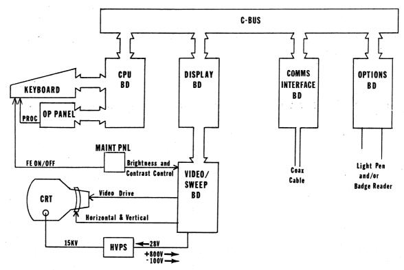
Figure 2.1 C277-III GENERAL BLOCK DIAGRAM
