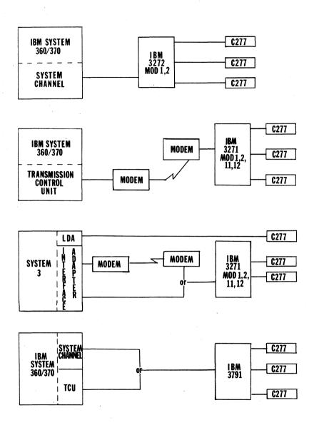
Figure 1.1 SYSTEM CONFIGURATOR
