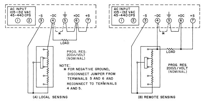
Figure 5. Programmed Voltage, with External Resistor
