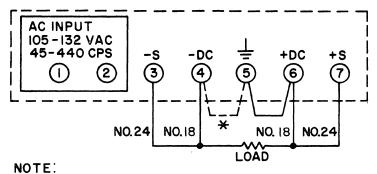
\* FOR NEGATIVE GROUND, DISCONNECT JUMPER FROM TERMINALS 5 AND 6 AND RECONNECT TO TERMINALS 4 AND 5.
