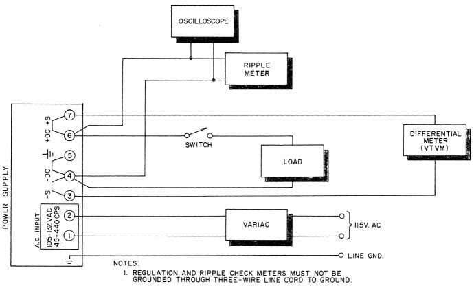
2. PERFORM CHECKS WITH LOCAL SENSING CONNECTIONS ONLY.
