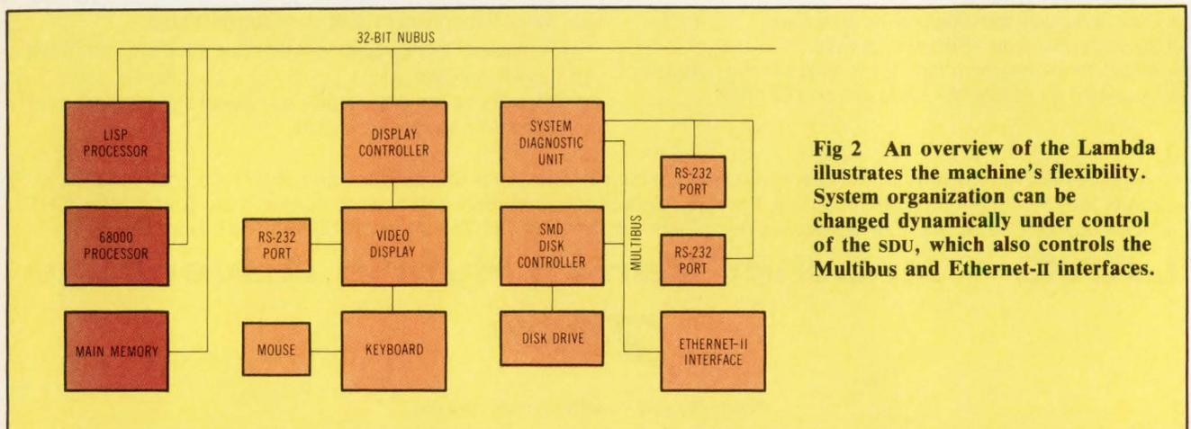
**Fig 2** An overview of the Lambda illustrates the machine's flexibility. System organization can be changed dynamically under control of the SDU, which also controls the Multibus and Ethernet-II interfaces.
