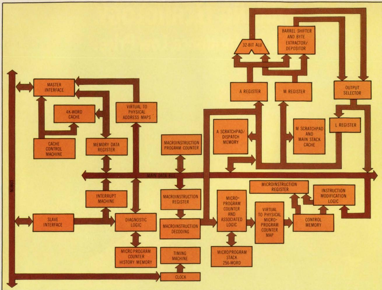
**Fig 3** The Lambda's Lisp processor consists of four boards (not outlined in this diagram). Clockwise from the top left are the memory interface board, which interacts with the NuBus; the data paths board, where data manipulation takes place; the control memory board, which contains the microcode functions; and the random gates board, which includes several control and diagnostic functions.
