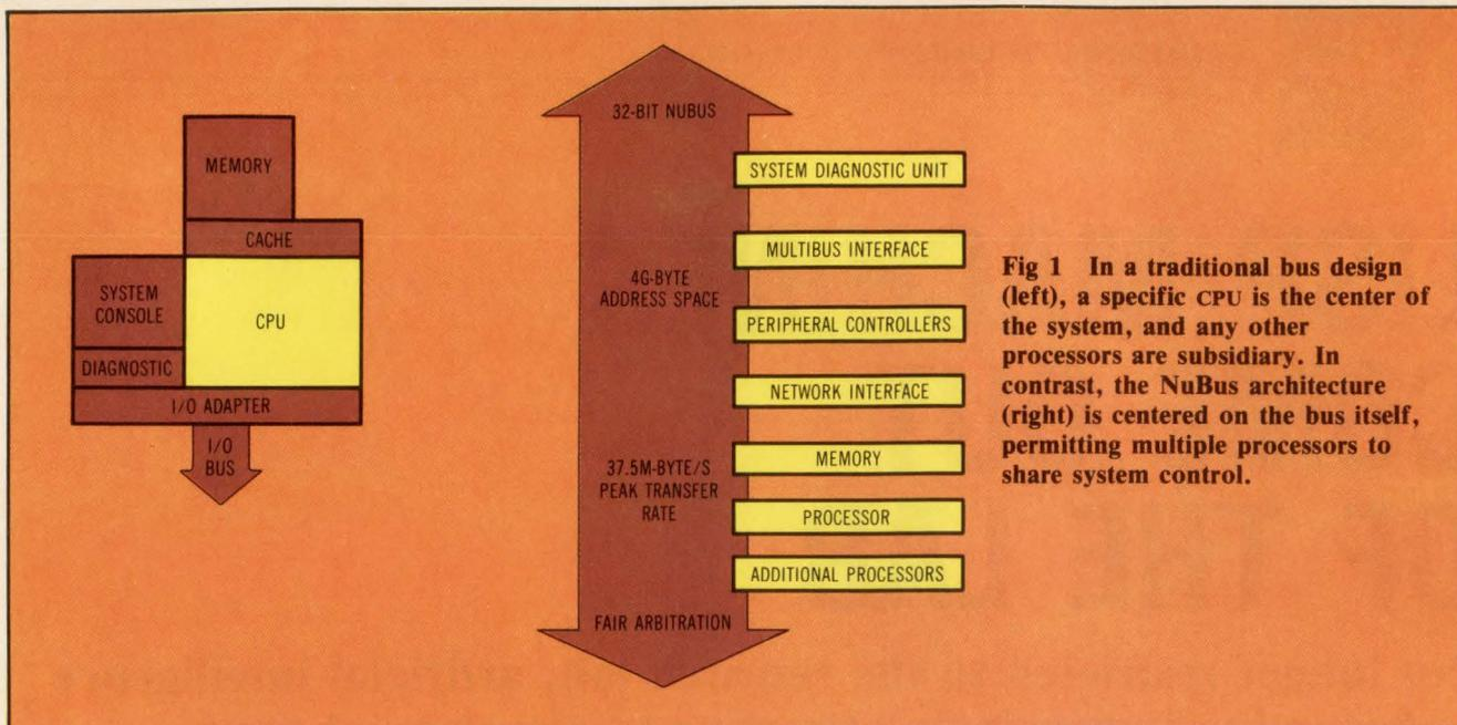
**Fig 1** In a traditional bus design (left), a specific CPU is the center of the system, and any other processors are subsidiary. In contrast, the NuBus architecture (right) is centered on the bus itself, permitting multiple processors to share system control.
