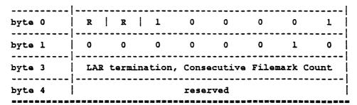
The value of byte 3 replaces the default count of 2 or any other value previously set. This is then used in any subsequent look-ahead-read operation to define the end of recorded data.
