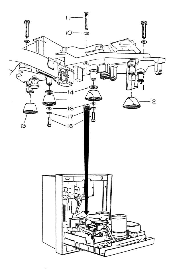
FIGURE 8.2.1 TAPE PATH ASSEMBLY
