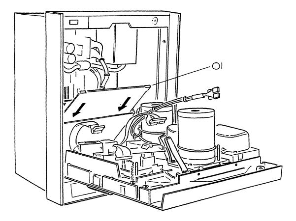
FIGURE 8.2.9 DATA CONTROL BOARD
