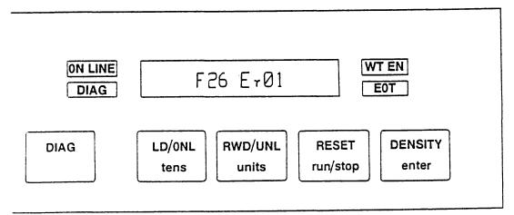
FIGURE 7.5.1 OPERATOR PANEL BUTTONS AND INDICATORS
