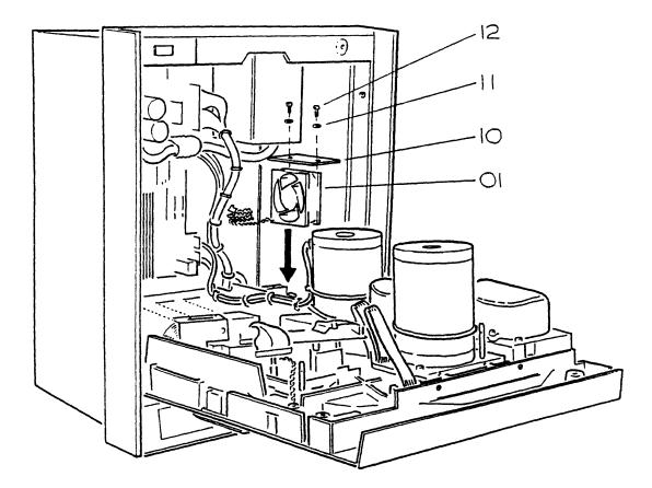
FIGURE 8.2.5 COOLING FAN ASSEMBLY
