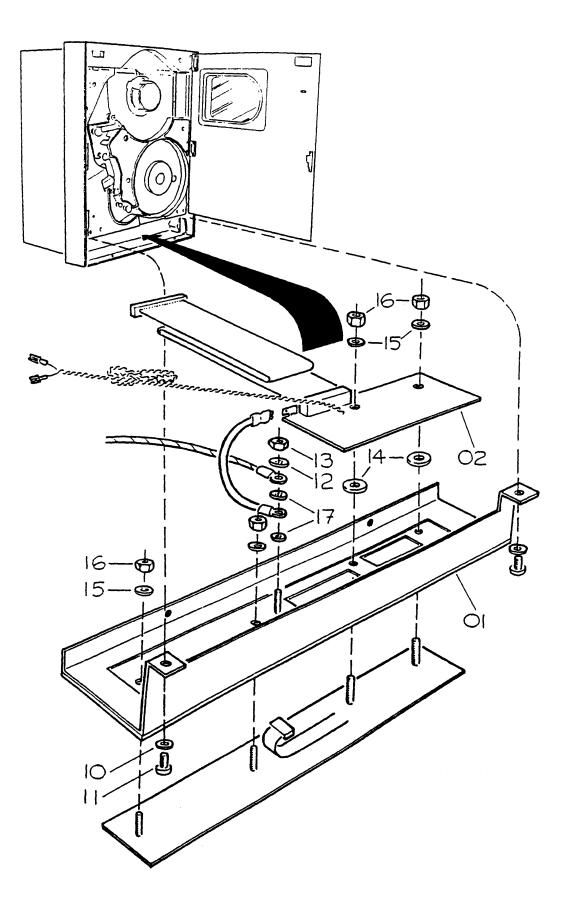
FIGURE 8.2.13 OPERATOR PANEL AND SWITCH FASCIA PCB
