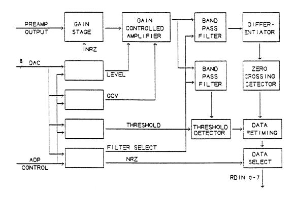
FIGURE 2.4.3.2(a) ADP READ BLOCK DIAGRAM - NRZ DENSITY
