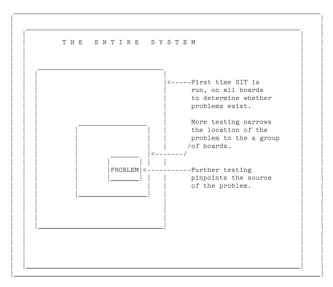
Figure 1-1. The Testing Procedure
