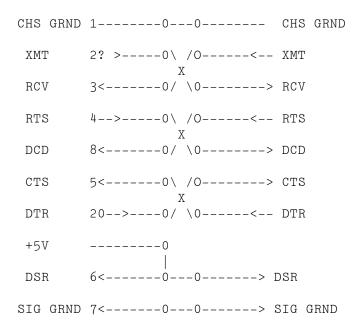
Figure 2-2. Standard Locally Connected Device Setup
