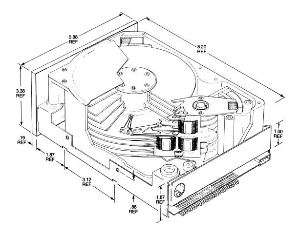
Figure 14-1 XT-3000 Mechanical Outline and Mounting Hole Location
