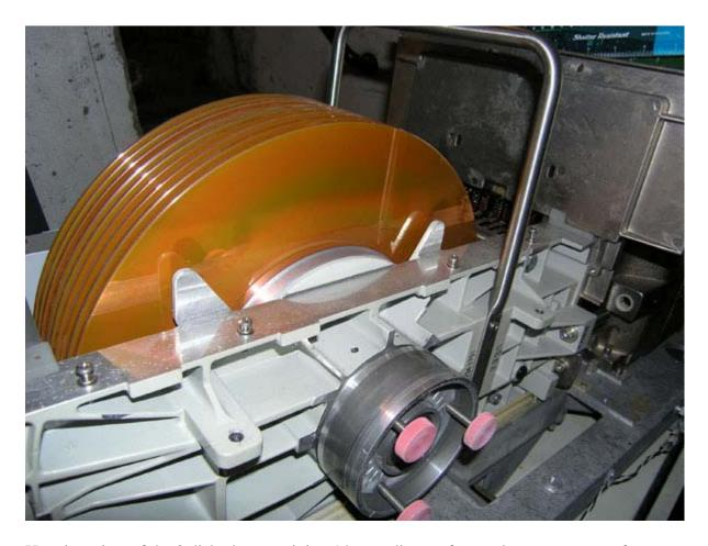
Here is a view of the 8 disk platters, giving 14 recording surfaces, plus two servo surfaces.
