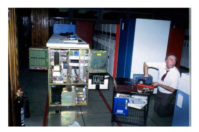
This is a photograph of a Memorex 3680 disk drive unit being repaired, as was too often the case. At the bottom is a power supply and out of sight, a large electric motor that turned the pack of disks via a belt. Above is control circuitry, and just visible a bit of the disk storage FRU itself.
