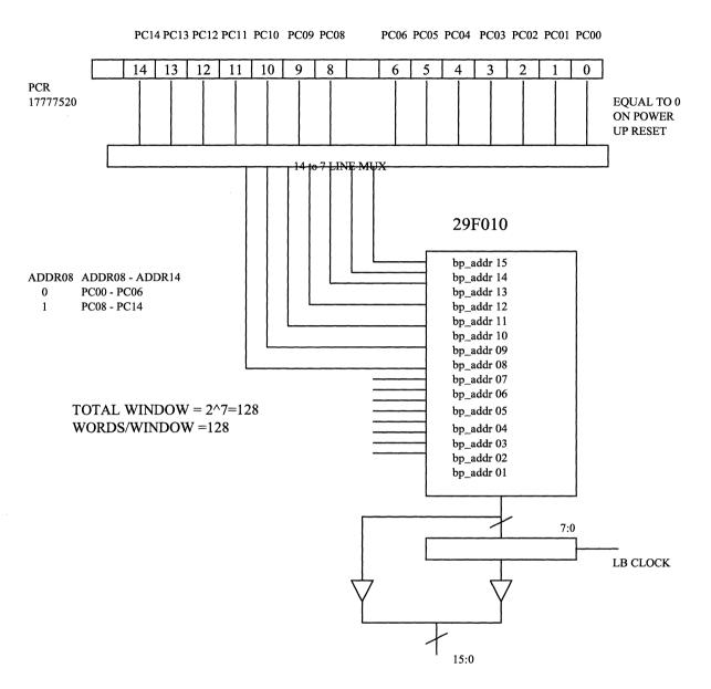
TOTAL BOOT CODE SPACE 128 WORDS X 127 WINDOWS = 31.75KBYTES. TOTAL SETUP ADDR. SPACE 128 BYTES X 1 = 128 BYTES.
