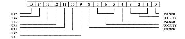
Figure 6.3 Program Interrupt Request Register.
