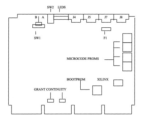
FIGURE 4.1 SBC M11 CONFIGURATION.
