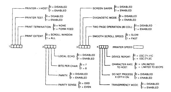
FIGURE 1.8.2 SET UP C SWITCHES
