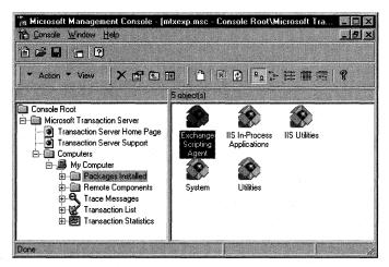
Figure 13-22. The Exchange Event Scripting Agent installed as an MTS component.
