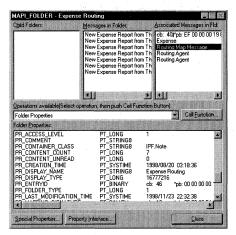
**Figure 16-1.** The MDB Viewer Test Application provides functionality to investigate the objects stored in your Exchange Server system. This tool can even be used to investigate the properties on rule items stored as hidden messages in your folders.
