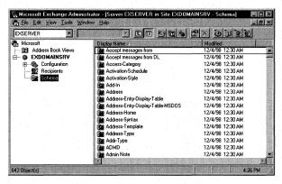
**Figure 15-1.** The Schema container in the Exchange Administrator program. You can search for attributes and classes defined by the Exchange Server schema using this view.
