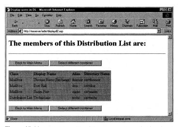
**Figure 15-11.** An HTML table of the users in a specific distribution list. The table is generated by parsing the return value of the Members method of the IADsGroup interface.
