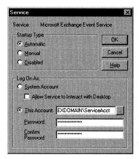
**Figure 13-2.** You change the Windows NT account that the Event Service runs under by using the Service applet in the Control Panel.
