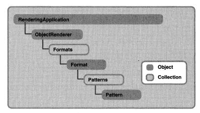
**Figure 12-31.** The ObjectRenderer object in the CDO Rendering library is used to display properties of individual items rather than of collections.
