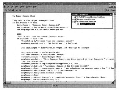
**Figure 13-9.** The Microsoft Script Debugger allows you to step through your scripts running on the Exchange server.
