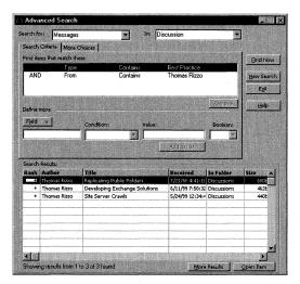
**Figure 17-11.** The COM add-in with multiple AND clauses and the results of the query in the Flexgrid control.
