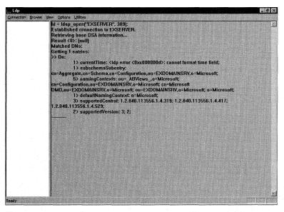
**Figure 15-17.** *IDP at work, connecting to an Exchange Server 5.5 directory. This tool is more low-level than the Active Directory Browser.*
