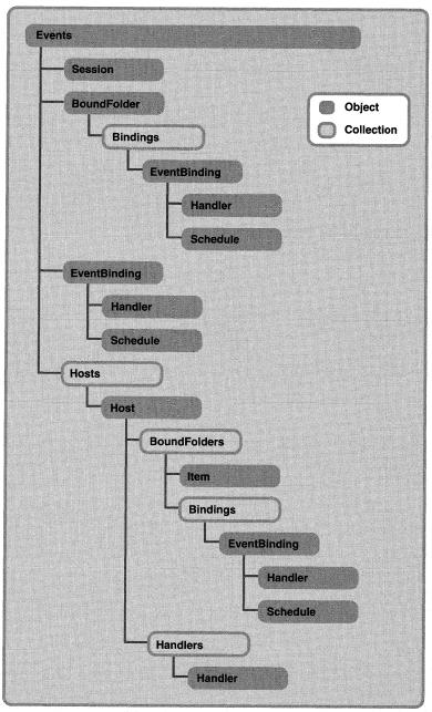
Figure 13-18. The object hierarchy for the Exchange Event Service Configuration library.
