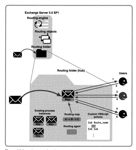
Figure 14-1. A diagram of Exchange Server routing.
