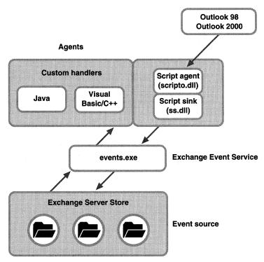
Figure 13-1. Architecture of the Exchange Event Service.
