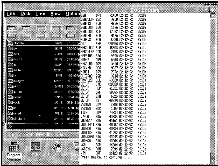
Figure 7-3: Configuring the number of screen lines for 50 instead of 25. A DIR command now shows a full 50 lines of a directory.
