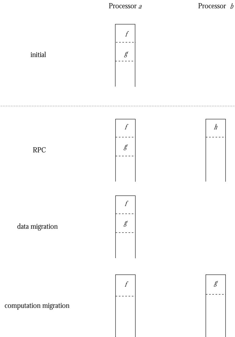
Figure 3-1. Stack patterns under different access mechanisms. Processor a is executing a thread, where f has called g . g is about to access remote data on processor b . Stacks grow downward in this figure.
