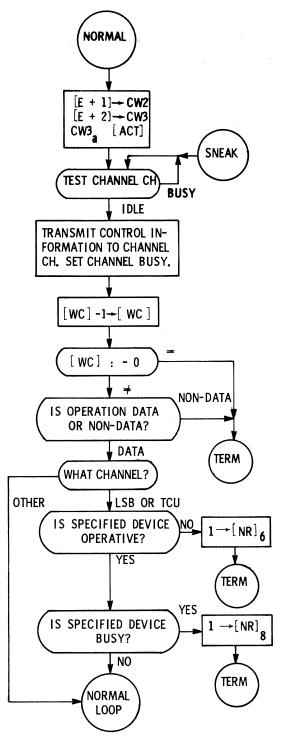
FETCH CONTROL WORD 2, DETERMINE IF OPERATION IS READ OR WRITE, OR NON-DATA. FETCH CONTROL WORD 3. EXTRACT BITS WHICH CONTROL BEHAVIOR OR ADDRESS COUNTER. EXTRACT CENTRAL MEMORY STARTING ADDRESS.
