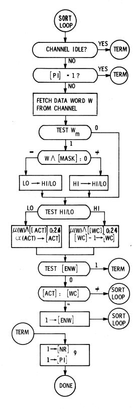
IF THE CHANNEL HAS BECOME IDLE, OR HAS INSTRUCTED PUP TO BECOME IDLE, OR CPS HAS INSTRUCTED PUP TO BECOME IDLE, THEN GO TERMINATE THE OPERATION.
