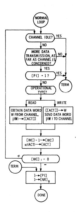
IF CHANNEL HAS BECOME IDLE, OR HAS INSTRUCTED PUP TO TERMINATE DATA TRANSMISSION, OR CPS HAS INSTRUCTED PUP TO BECOME IDLE, THEN GO TERMINATE THE OPERATION.
